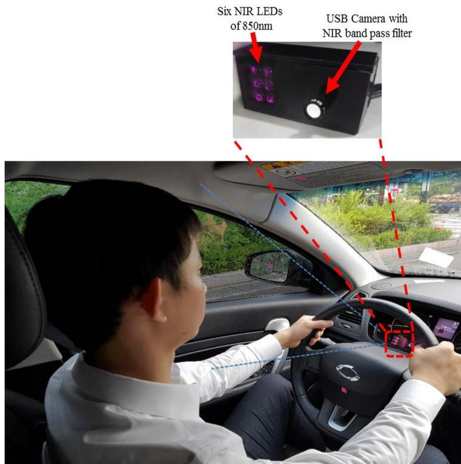
**Figure 2.** Experimental environment and proposed gaze detection system in vehicle environment.
