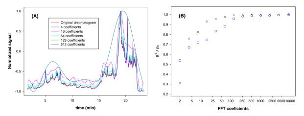
**Fig. S1.** Selection of the optimal number of Fourier coefficients for signal compression. Changes in (A) chromatogram reconstruction and (B)  $R^2$  and *fc* coefficients depending on the number of coefficients considered.
