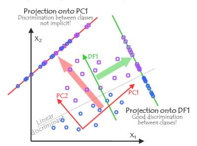
**Fig. S2.** Schematic comparison between PCA and LDA. Briefly, PCA seeks for the direction of maximum variance between the variables, while LDA seeks for the direction that provides maximum separation between the classes. Note also that in PCA as many new PCs as variables in the original data are obtained, whereas in LDA only as many #groups-1 DFs are obtained. Adapted from Cetó, X., *et al.* Electroanalysis, 25 (2013), 1635.
