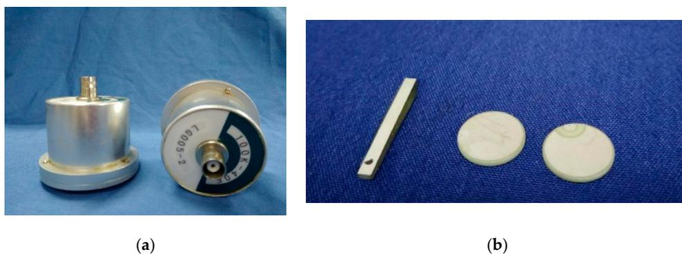
**Figure 7.** The transducers used in the detecting system. (a) Ultrasonic probe. (b) piezoceramic transducers.
