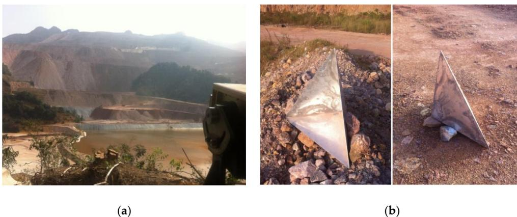
**Figure 8.** Deformation monitoring for case study 2: (a) the monitoring scene and (b) corner reflectors.
