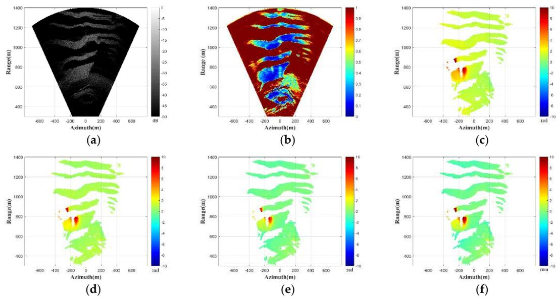
**Figure 9.** Experimental results: (a) reflectivity image; (b) sub-images entropy map; (c) uncorrected phase; (d) corrected phases using the linear model method; (e) corrected phase using proposed method; and (f) deformation map.
