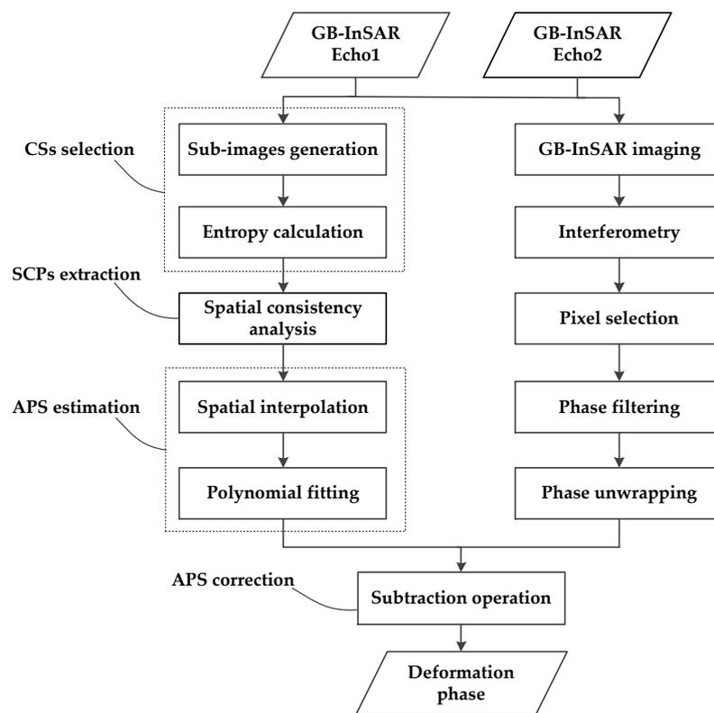
Figure 4. Time- and space-varying atmospheric phase correction algorithm flowchart.
