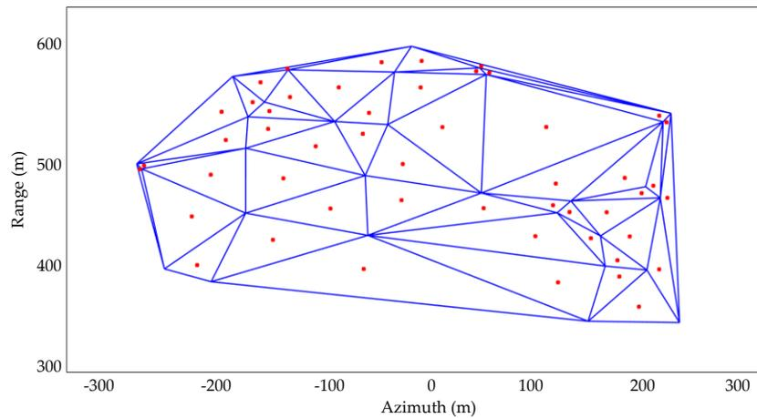
**Figure 3.** Diagrammatic sketch of Delaunay triangulation. The red points are the pending interpolation points.
