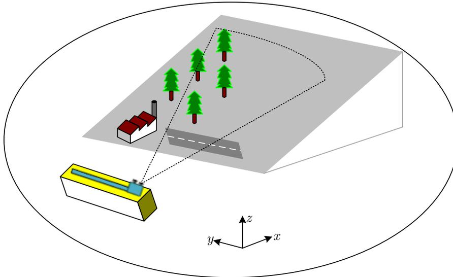
**Figure 1.** Observation geometry of ground-based synthetic aperture radar (GB-SAR).
