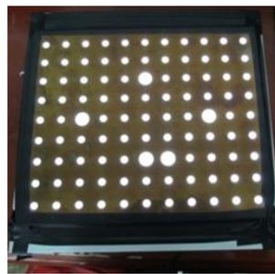
Figure 6. Target for binocular vision calibration.
