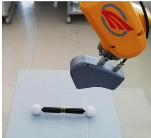
Figure 15. The measurement of ball arm by AASM.
