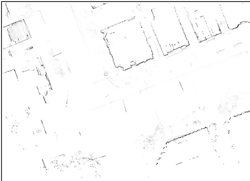
**Figure 15.** Probabilistic occupancy grid map generated by applying the IEPF algorithm.
