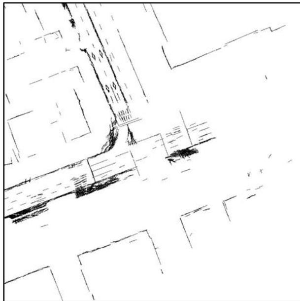
Figure 20. Result of converting Figure 19 into occupancy grid map.
