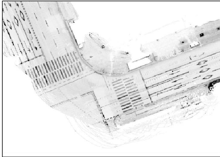
Figure 6. Generated road reflectivity map (before plane extraction).
