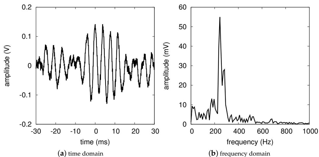
**Figure 6.** People detection results. (a) Time domain output signal corresponding to a person at a 6-m distance with a relative speed of about 1.5 m/s. (b) Frequency domain output signal obtained performing the FFT of panel (a). The main peak corresponds to a Doppler frequency of 244 Hz.
