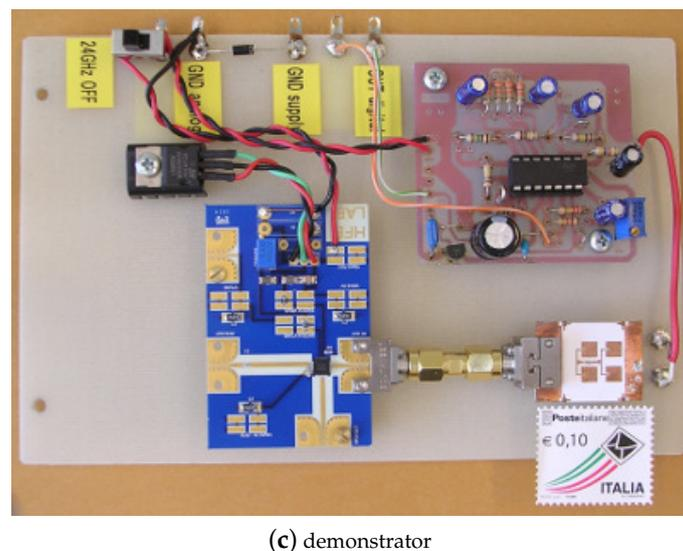
**Figure 4.** Fabricated 24-GHz front-end on a multi-layer cellulose-based substrate. (a) Antenna side. (b) Active circuit side. (c) Demonstrator including external VCO, intermediate frequency (IF) amplification and triggering stages. The used substrate area is  $20 \times 27 \text{ mm}^2$ . The realized cellulose circuit has the size of a postage stamp.
