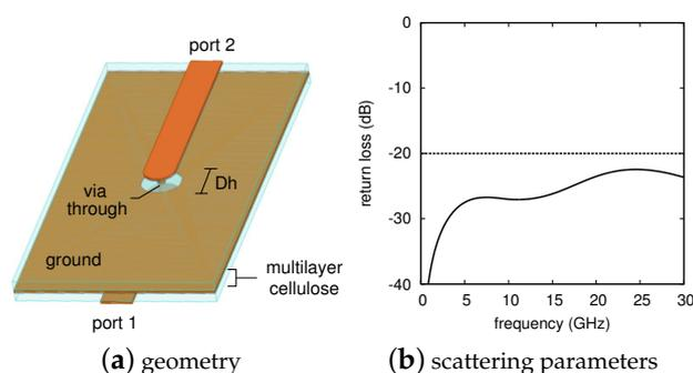
**Figure A1.** Via-through connection in a multilayer cellulose circuit: structure (a) and simulated scattering parameters (b). The main geometrical parameters are the hole diameter  $D_h = 1.05$  mm, and via diameter of 0.2 mm.
