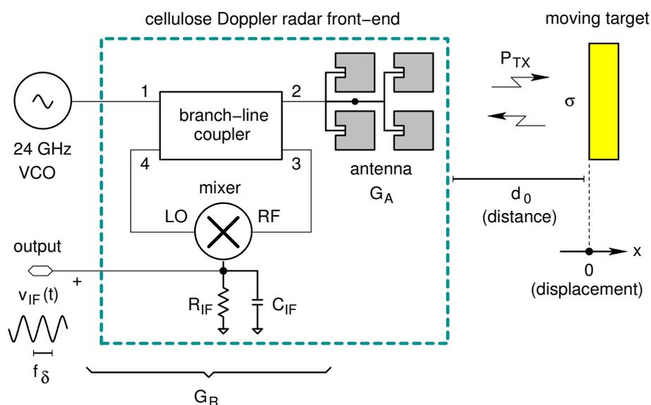
**Figure 1.** Block diagram of the radar sensor. The circuit uses a branch-line power divider to couple the voltage-controlled oscillator (VCO) to both the antenna and the mixer. If the target moves, a Doppler frequency shift  $f_\delta$  is produced in the reflected wave and is detected by the mixer circuit. The resistance  $R_{IF}$  and the capacitor  $C_{IF}$  constitute a low-pass filter and terminate the mixer output port. LO: local oscillator; RF: radio frequency.
