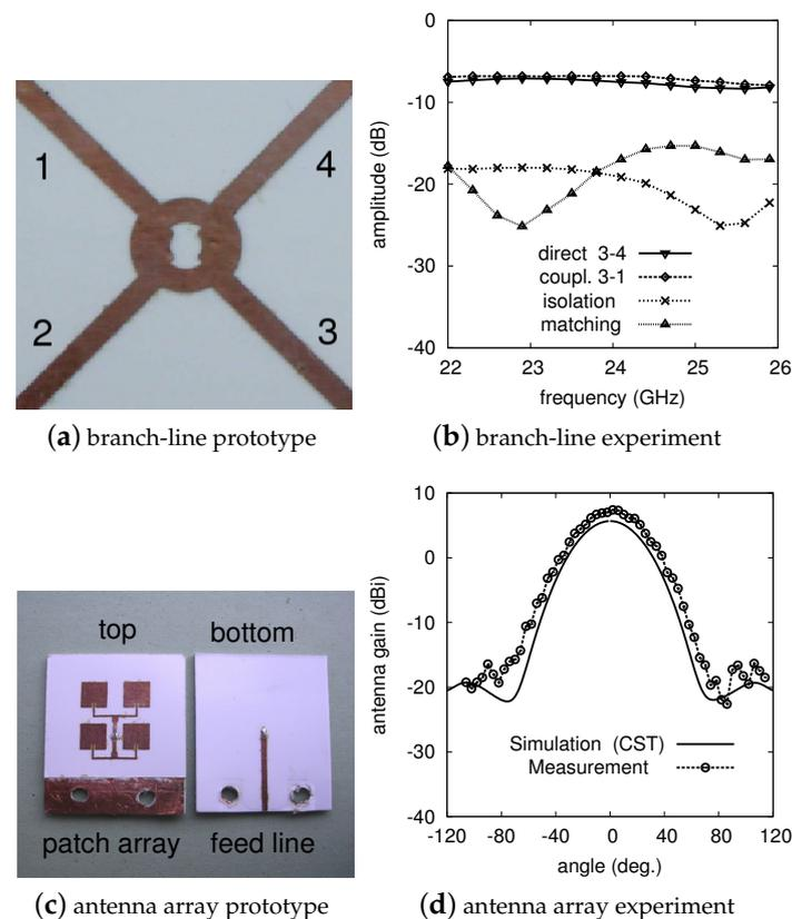
**Figure A2.** Branch-line coupler and patch antenna array. Branch-line: manufactured prototype (a) and experimental results (b). The coupler diameter is about 4.4 mm. After Reference [39]. Antenna array: manufactured prototype (c) and experimental results (d). The antenna dimensions are  $20 \times 20 \text{ mm}^2$ . After Reference [40].
