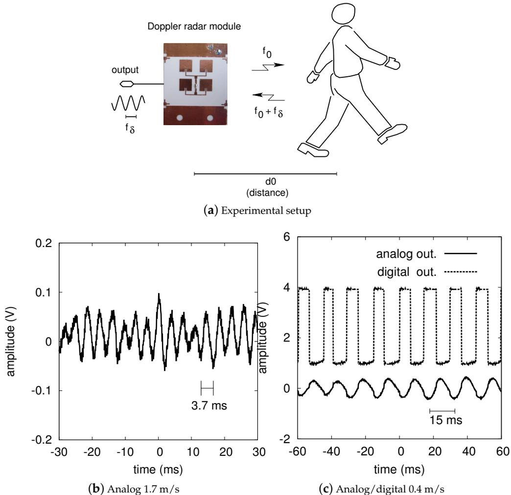
**Figure 5.** People detection results. (a) Experimental setup. (b) Analog output corresponding to a person at an 8-m distance with a relative speed of 1.7 m/s. (c) Analog and digital outputs associated to a person at a 3-m distance that slowly moves. In the last case the relative speed is of only 0.4 m/s. These signals are measured after the amplification and, possibly, after the triggering stages of the demonstrator (see Figure 4).
