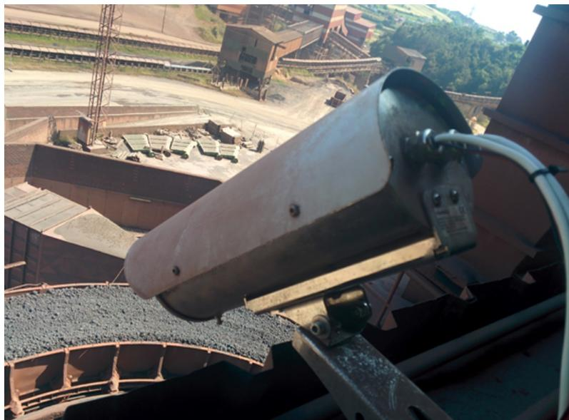
**Figure 13.** Infrared camera for sinter monitoring.
