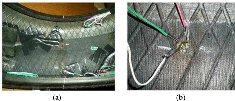
Figure 3. (a) Strain gauges' setup; (b) Multiaxial gauge example.
