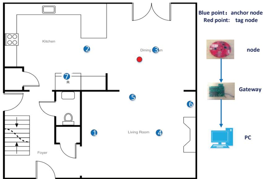
**Figure 4.** The diagram of the sensor deployment.
