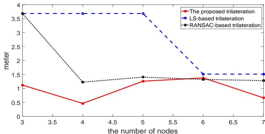
**Figure 8.** Comparison of RMSE varying with numbers of sensors among the proposed method, the LS-based trilateration method and the RANSAC-based method.
