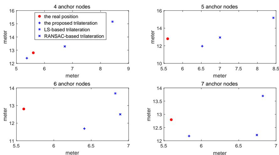
**Figure 7.** Comparison of the estimated location among the proposed method, the LS-based trilateration method and the RANSAC-based method.**Table 2.** Comparison of RMSE among the proposed method, the LS-based trilateration method and the RANSAC-based method (m).
