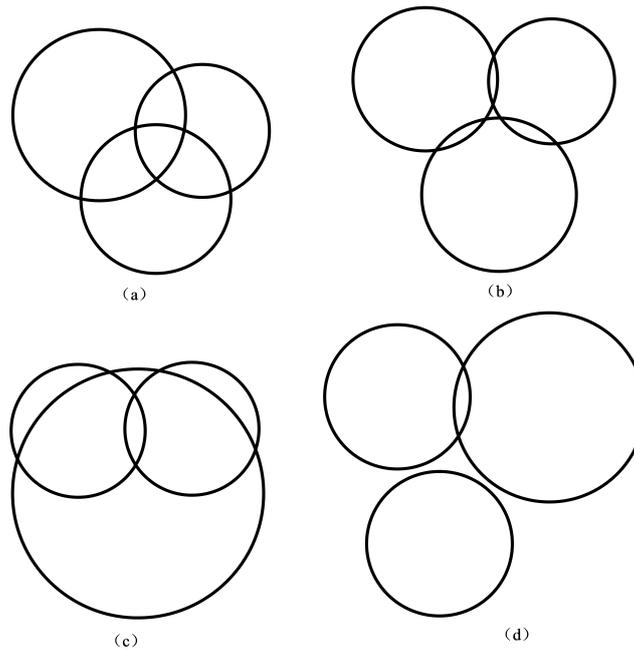
**Figure 1.** The diagrams of all possibilities of intersections of anchor circles influenced by noise. (a) diagram of two intersection points, one of which is outside and one of which is inside of the third circle; (b) diagram of two intersection points, both of which are outside of the third circle; (c) diagram of two intersection points, both of which are inside of the third circle; and (d) diagram of no intersection points.
