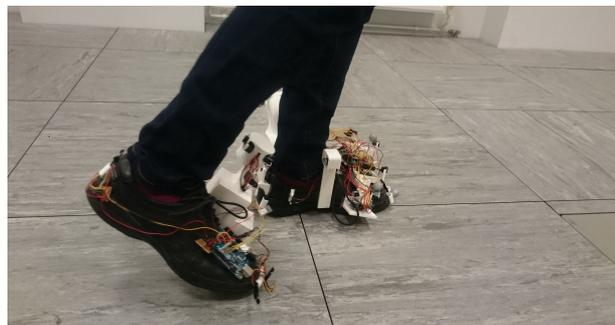
**Figure 5.** The wearable sensing system during Type 1 walking. The left foot is on the ground when the zero-velocity updates (ZUPT) and Heuristic Drift Reduction (HDR) corrections are applied.
