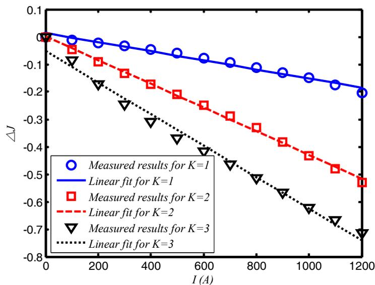
**Figure 4.** The relationship between current and the normalized output light difference  $\Delta J$ . The linear fits are based on the least squares method.
