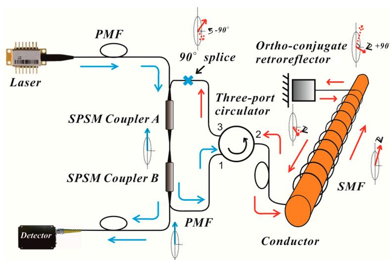
Figure 1. The configuration of the loop AFCS based on SPSM couplers.
