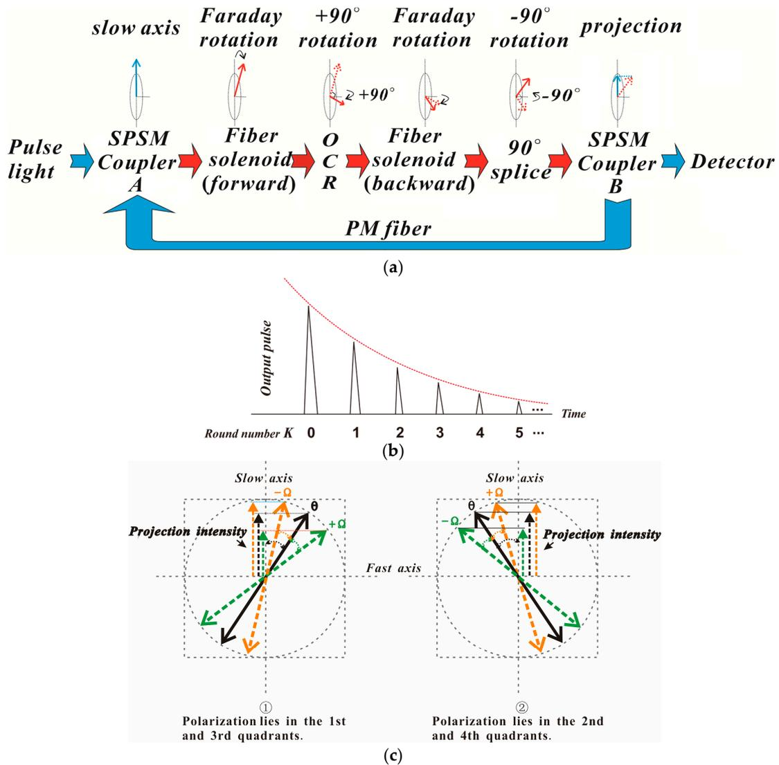
**Figure 2.** The changing process of light in the loop AFCS based on the SPSM coupler, (a) for the change of polarization state of light; (b) for the output signal; and (c) for the relationship between Faraday rotation angle  $\Omega$  and the angle  $\theta$ .
