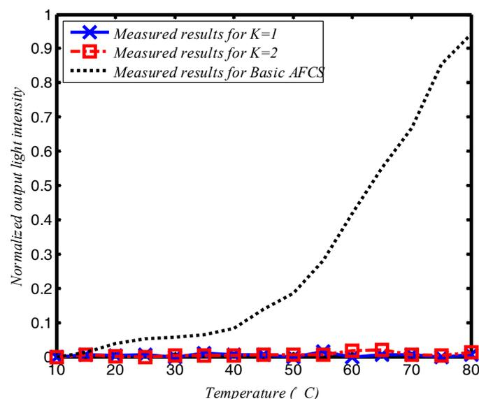
Figure 5. The effect of temperature on the loop AFCS based on the SPSM couplers.
