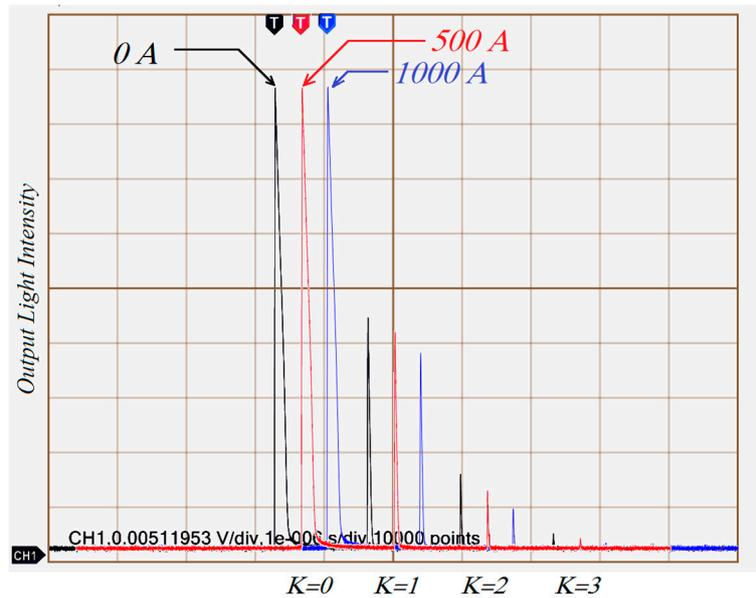
**Figure 3.** Intensity variations of output light for currents of 0 A, 500 A, and 1000 A passing through the sensor head. Measurements were carried out with a Tektronix TDS3054B 500 digital oscilloscope.
