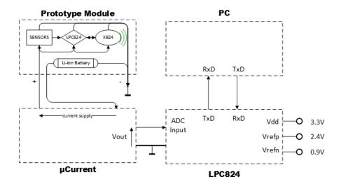
**Figure 6.** Experimental energy measuring schema is measured converting the current into voltage with the  $\mu$  Current device and using it as the input of the LPC824's ADC to be calculated with a PC.
