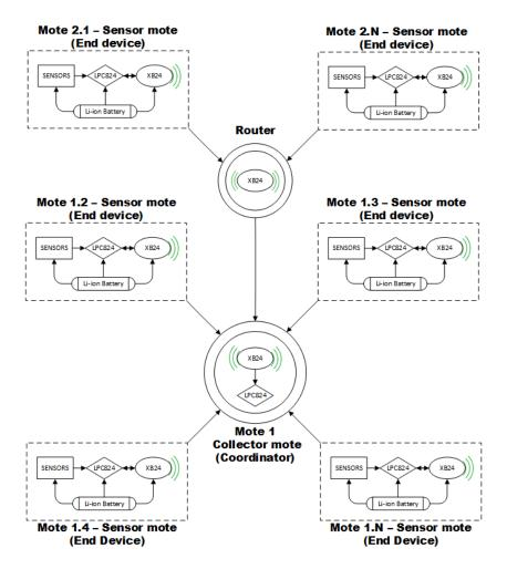
**Figure 1.** Reference Framework. It is composed of the collector mote, the router motes and the sensor motes. The sensor motes send the data information to the collector and then the collector processes it.
