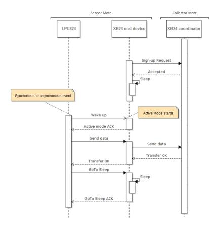
**Figure 4.** Sequence diagram of LOw power Konsumption Algorithm (LOKA) to reduce consumption in a sensor mote. It is divided into three columns that correspond to the execution flow of the LPC824 program, the XB24 end-device program and the XB24 coordinator program.
