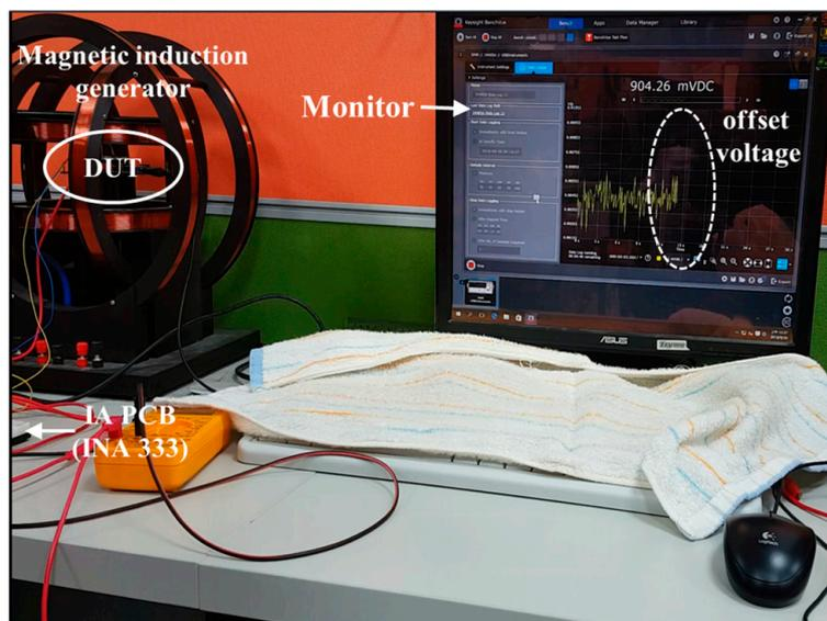
Figure 6. Offset voltage (right circle) displayed on the monitor without a magnetic body and DUT (Device under test) placed in the magnetic induction generator.
