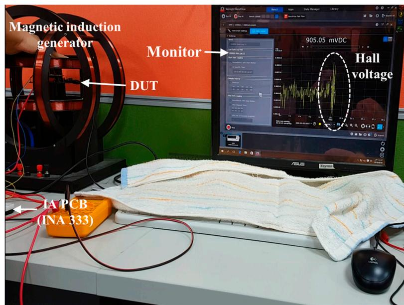
**Figure 7.** Hall voltage appears on the monitor evidently when the magnetic body comes in contact with the distance detector.
