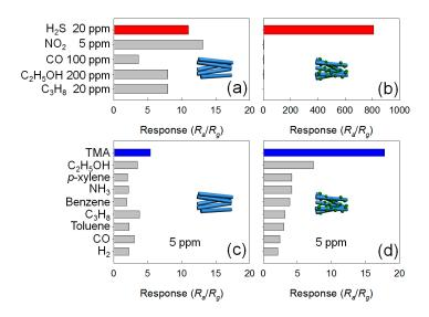
**Figure 4.** Gas selectivity of (a) pristine  $SnO_2$  NW network sensor and (b) CuO-decorated  $SnO_2$  NW network sensors at 300 °C; gas selectivity of (c) pristine ZnO NW network sensor and (d)  $Cr_2O_3$ -decorated ZnO NW network sensor at 400 °C. Adapted from [80,91] with permission; (a,b) [91] Copyright (2009) Elsevier; (c,d) [80] Copyright (2012) IOP Publishing Ltd.
