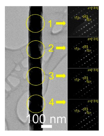
**Figure 9.** TEM image and selected area electron diffraction (SAED) patterns for the  $Mn_3O_4$  NW. Reprinted from [84] with permission. Copyright (2012) American Chemical Society.
