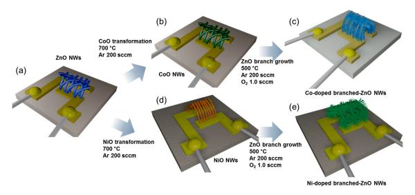
**Figure 10.** (a) Growth of ZnO NWs on alumina substrate with Au electrodes; (b) transformation of ZnO NWs into CoO NWs; (c) growth of Co-doped branched ZnO NWs from CoO NWs; (d) transformation of ZnO NWs into NiO NWs; (e) growth of Ni-doped ZnO NWs from NiO NWs. Reproduced from [131,137] with permission; (a–c) [137] Copyright (2014) American Chemical Society; (d,e) [131] Copyright (2015) Elsevier.
