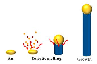
Figure 1. Schematic illustration of the vapor-liquid-solid mechanism.
