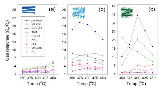
**Figure 11.** Gas response of (a) pristine ZnO; (b) Co-doped branched ZnO NWs; and (c) Ni-doped branched ZnO NWs to 5 ppm p-xylene, toluene,  $C_2H_5OH$ , TMA, HCHO, NH<sub>3</sub>, CO, benzene, and H<sub>2</sub> at 350–450 °C. Reproduced from [131,137] with permission; (a,b) [137] Copyright (2014) American Chemical Society; (c) [131] Copyright (2015) Elsevier.
