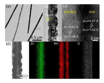
**Figure 8.** Morphologies and crystal structures of ZnO-ZnMn $_2$ O $_4$  NCs: (a,b) TEM images of ZnO-ZnMn $_2$ O $_4$  NCs grown on Si substrates; (c) Lattice-resolved image of ZnO-ZnMn $_2$ O $_4$  NCs; (d) Energy dispersive X-ray spectroscopy (EDS) elemental mapping of Zn, Mn, and O. Reprinted from [84] with permission. Copyright (2012) American Chemical Society.
