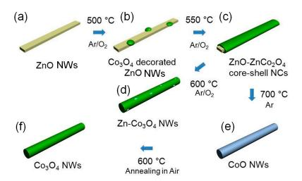
**Figure 7.** A schematic illustration of the transformation from ZnO NW to CoO NW and  $Co_3O_4$  NW. Adapted from [105] with permission. Copyright (2012) The Royal Society of Chemistry.
