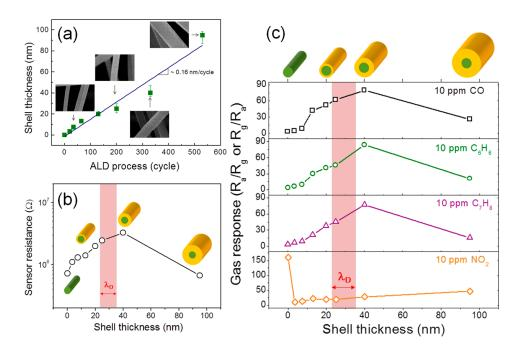
**Figure 6.** (a) Relationship between ZnO shell thickness and number of atomic layer deposition (ALD) cycles; (b) sensor resistance in air and (c) gas responses of SnO<sub>2</sub>-ZnO core-shell NWs as a function of ZnO shell thickness. Reprinted from [104] with permission. Copyright (2014) American Chemical Society.
