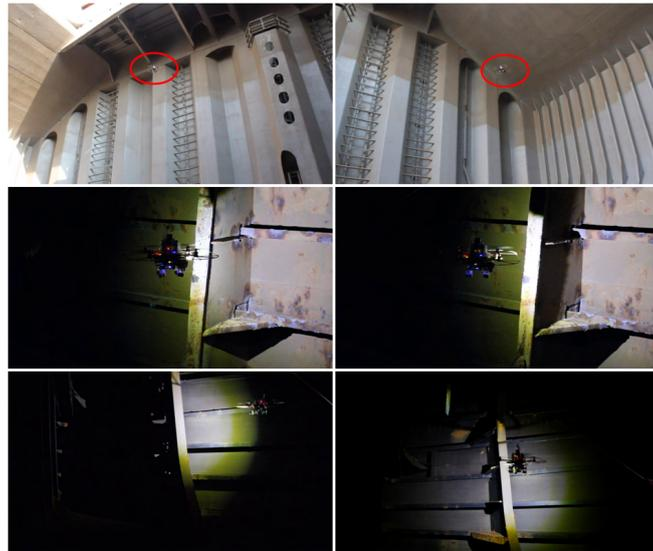
**Figure 19.** Pictures from some of the flights performed inside the bulk carrier: (**Top**) cargo hold; (**Middle**) top-side tank; (**Bottom**) fore-peak tank.
