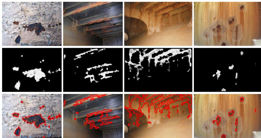
**Figure 14.** Examples of CBC detection for the *generic corrosion* dataset (I): **(Top)** original images; **(Middle)** CBC detector output; **(Bottom)** detection contours superimposed in red.
