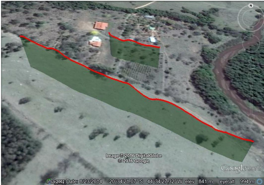
**Figure 10.** Hill flight path from GPS data of the telemetry logs. This image is from a perspective view, where the red lines represent the flight paths of the two areas of interest and the green shade the projection of this flight path on the Earth’s surface.
