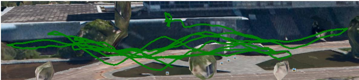
Figure 14. Manual flight path with vertical zig-zag pattern.
