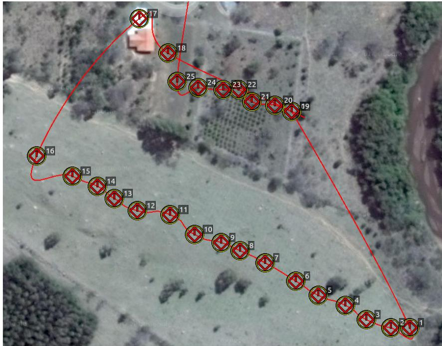
**Figure 8.** Hill flight plan. The figure shows the flight plan for the hill video sequence: the first slope is between Waypoints 1 and 16 and the second between Waypoints 19 and 25.
