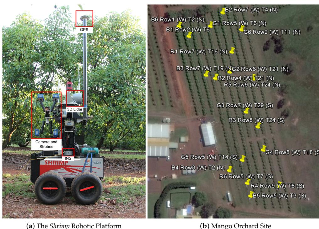
**Figure 2.** The robotic platform Shrimp (a) with labels to indicate the locations of the sensors used in this paper; a map of the mango orchard test block (b), with yellow pins marking the 18 trees that were selected for ground-truth field and harvest fruit counts.
