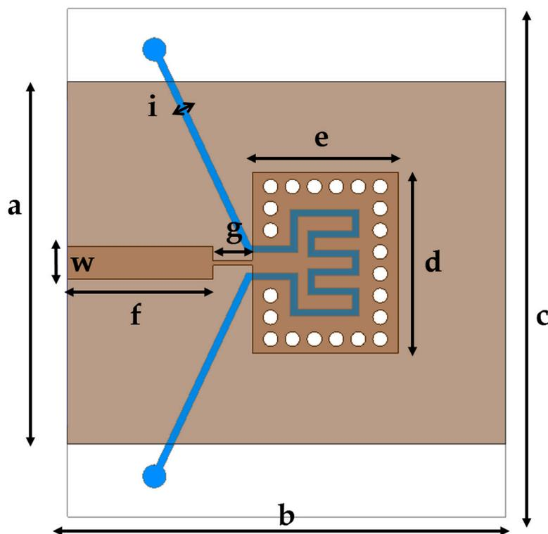
Figure 4. Proposed SIW chemical sensor (top view).
