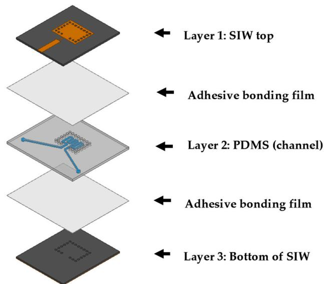
Figure 3. Layers of the proposed SIW chemical sensor.
