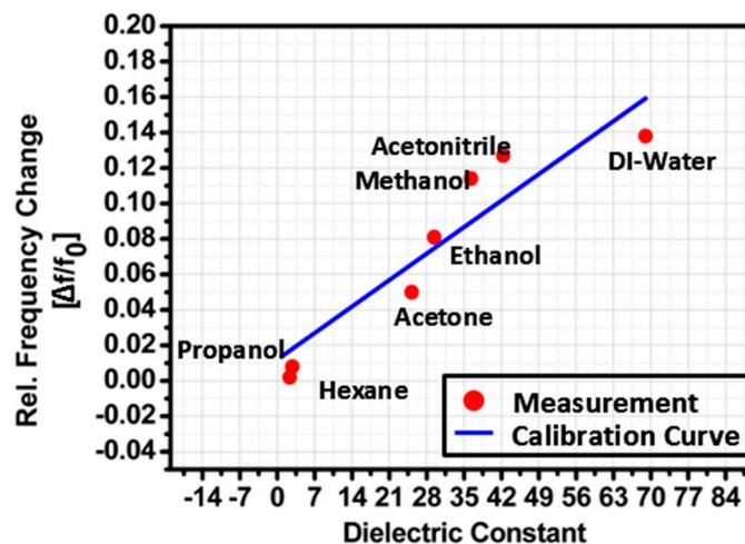
Figure 9. Sensitivity of the proposed SIW chemical sensor.
