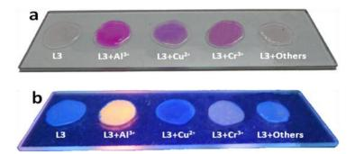
Figure 11. Photographs of ligand doped PVC polymeric thin films under visible (a) and fluorescent light (b).
