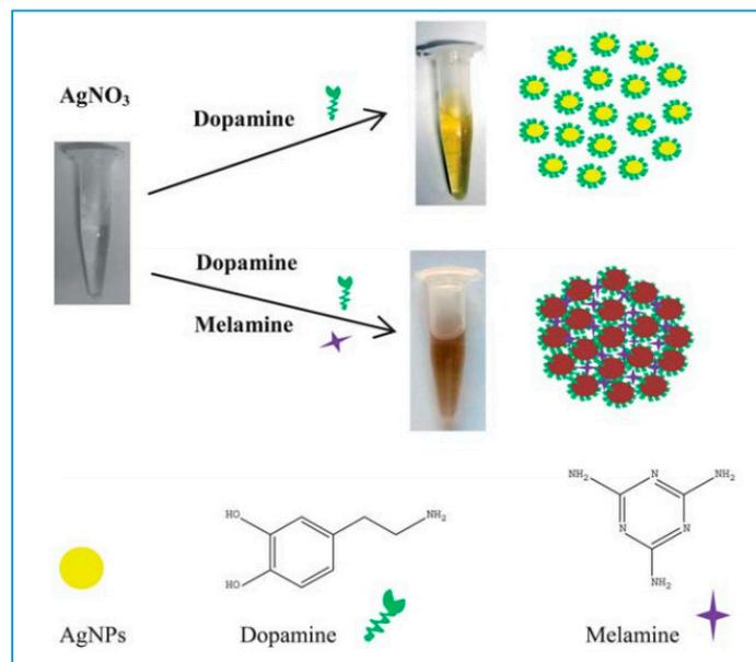
**Figure 2.** Schematic illustration of colorimetric method with AgNPs/dopamine system for the detection of melamine (reproduced from [48] with permission of The Royal Society of Chemistry).
