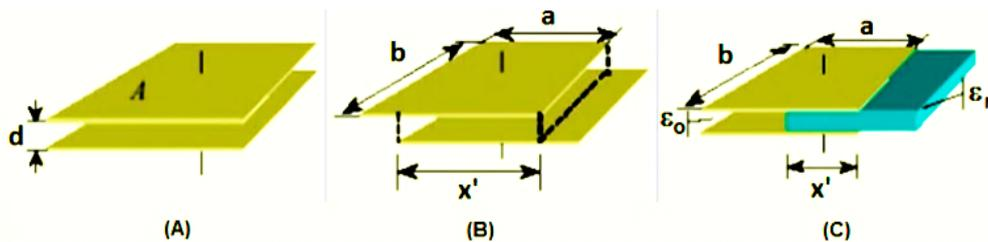
**Figure 1.** Illustration of a Capacitive Sensor of Parallel Plates, where (a) indicates a possible variation in the distance between the plates; (b) indicates a possible variation of the common surface; and (c) the alteration of the dielectric element.
