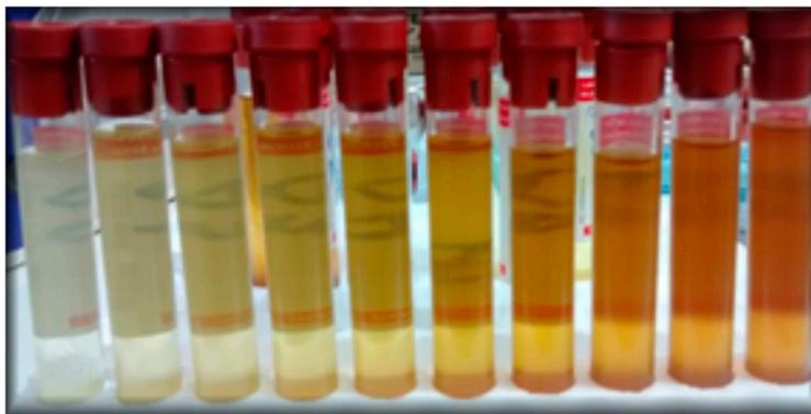
**Figure 6.** Changes in coloration of oil samples collected after each heating and cooling cycle.
