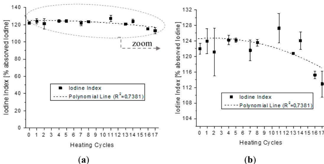
**Figure 12.** Value of the iodine index at 20 °C, for each one of the seventeen consecutive heating cycles, (a) in full scale; and (b) zoom on measurement values.
