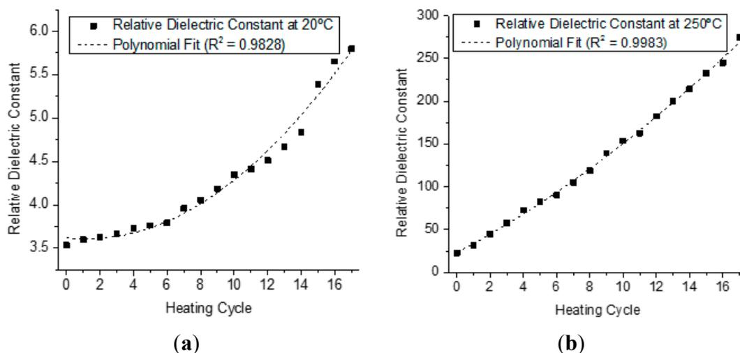
**Figure 9.** Value of the Dielectric Constant at 20 °C in (a) and at 250 °C in (b), obtained after each one of the seventeen consecutive heating cycles of the soybean oil samples.
