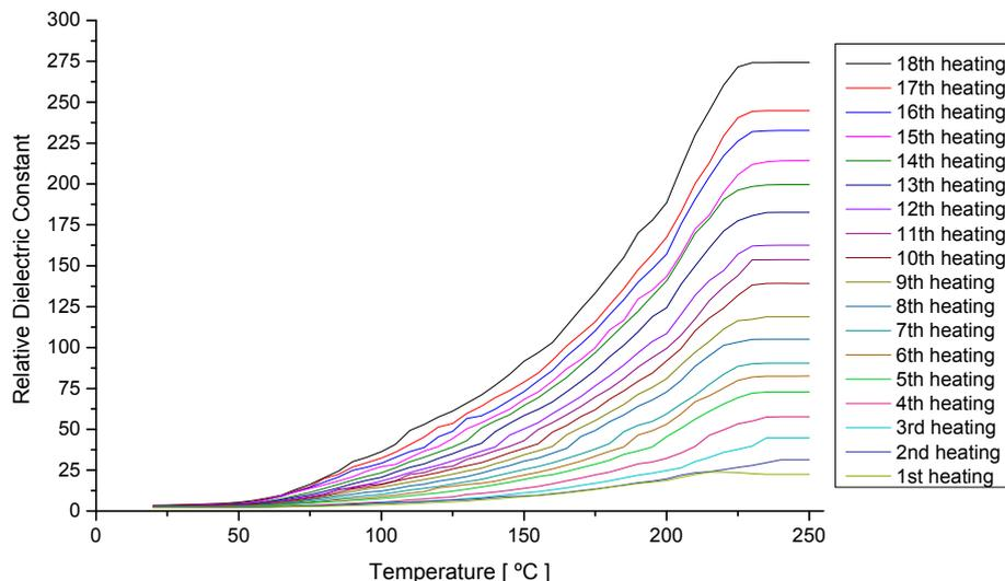
**Figure 8.** Variation of the Dielectric Constant in relation to the temperature during eighteen heating cycles of a sample of soybean oil (20 to 250 °C).
