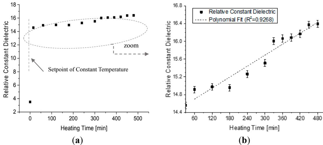
**Figure 7.** Variation of the Dielectric Constant in relation to time for a soybean oil sample kept at the constant temperature of 180 °C. (a) Experimental data of all the heating process since 20 °C; and (b) zoom of the data after setpoint of constant temperature.
