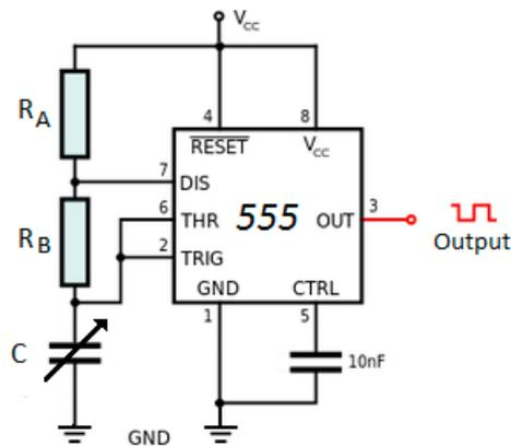
**Figure 4.** Astable vibrator based on the CI CA555 with frequency depending on a capacitive sensor [16].
