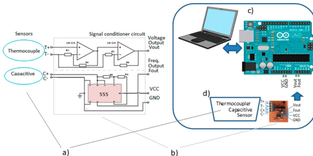
**Figure 5.** Data acquisition system of the sensors. (a) capacitive and temperature sensors; (b) Signal conditioner circuit; (c) system for storing data; and (d) recipient of oil sample.
