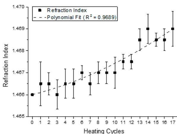
**Figure 11.** Value of the refraction index at 20 °C, for each one of the consecutive heating cycles.
