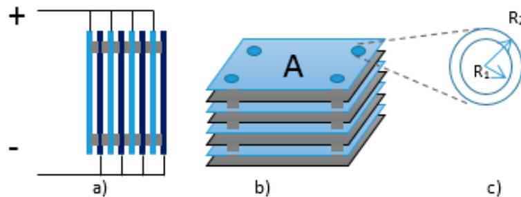
**Figure 2.** Outline of the capacitive sensor's prototype. (a) Side view; (b) Perspective view; and (c) Circular dielectric insulators with internal ( $R_1$ ) and external ( $R_2$ ) radius.
