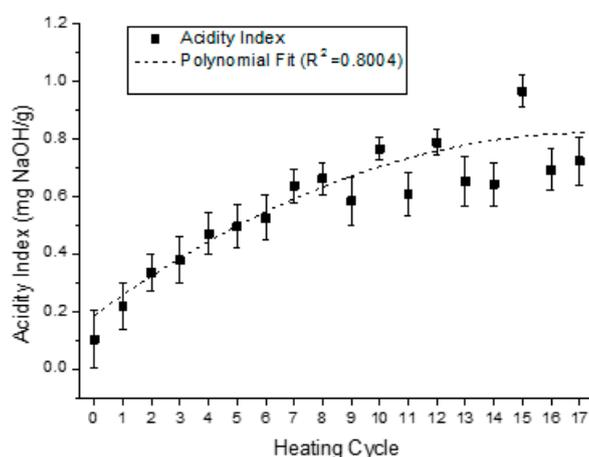
**Figure 10.** Variation of the acidity index at 20 °C, for each one of the eighteen heating cycles.
