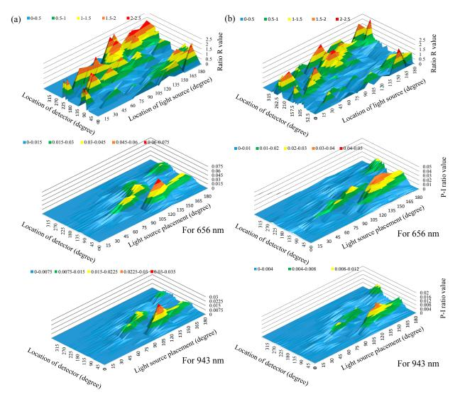
**Figure 5.** Comparisons of simulation results for the P-I ratio value and ratio R value by using a single detector and a multi-detector when the light source was placed at (a) 135°, (b) 150° and (c) 165°, respectively.
