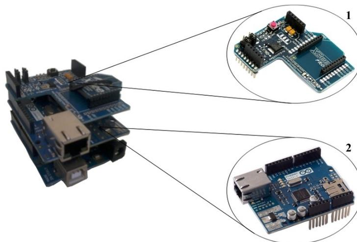
As the designed gateway needs to communicate with several XBee modules and also have access to an Ethernet network, we needed to enhance the typical Arduino by using shields. Therefore, two shields were employed (one XBee and one Ethernet shield) to allow the connection between the WSN and the cloud server. Thereafter, the XBee shield (Label 1, Figure 3) receives the gathered data from the WSN and transmits it by means of the Ethernet shield (Label 2, Figure 3) to a cloud server.
