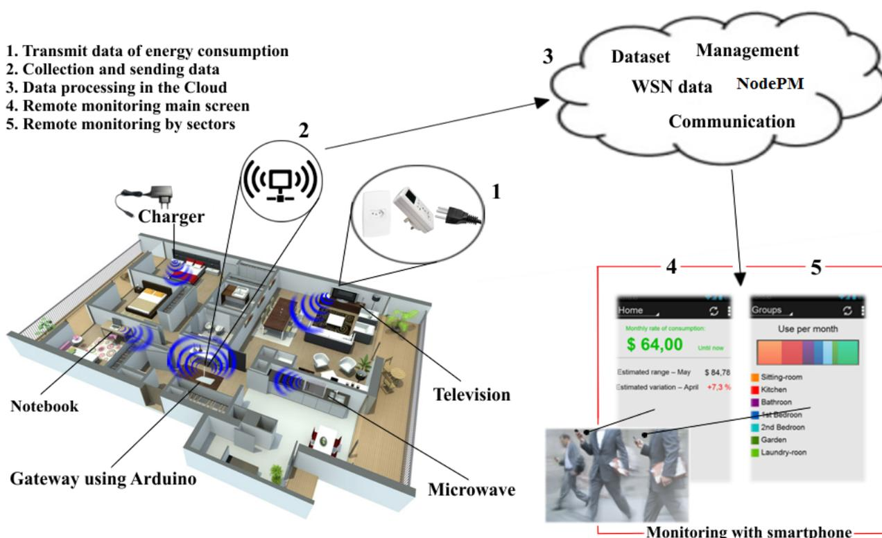
As a result, the user receives the alerts and can visualize the most important information about energy consumption, as presented in Label 4 of Figure 1. The monitoring of the sectors (Label 5, Figure 1) is carried out with regard to the equipment and the room in the house, and/or any area being used, and is only possible on account of the WSN.
