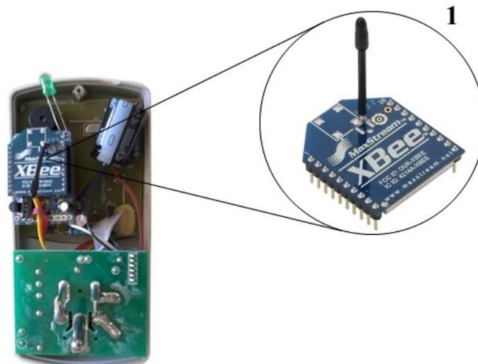
The choice of the communication module used in the wattmeter (Model XB24-AWI-001) can be explained by the following reasons: (i) low energy consumption; and (ii) an average reach area of 40 m indoors and/or 120 m outdoors.
