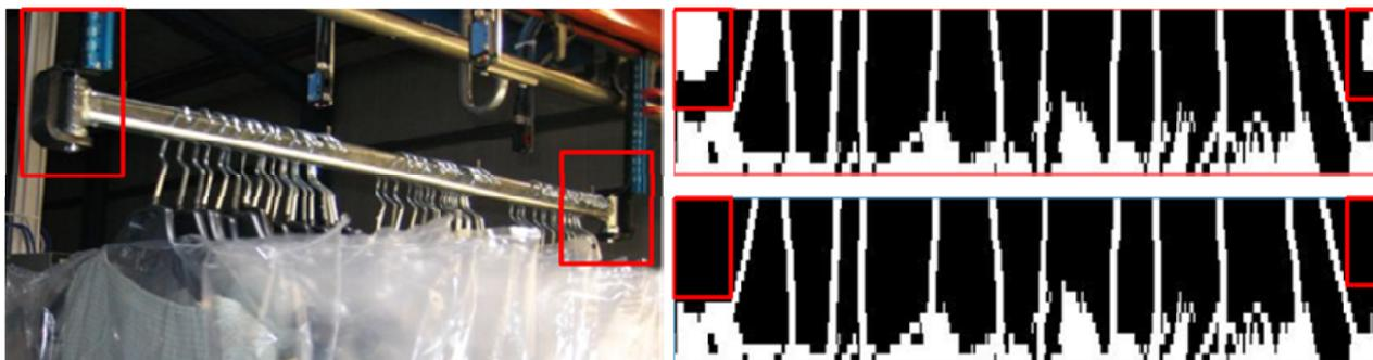
The purpose of the image processing is to isolate the visible area of the hanger hooks and to identify the characteristic pattern of a hanger [17]. In practice, there is a great variety of cases and problems to identify patterns of hangers (see Figure 9); though, they are identical in either trolley or continuous chain mode:
