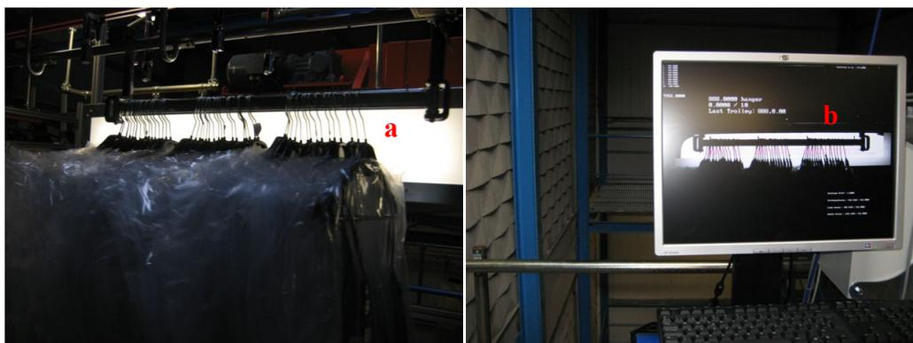
Our solution, on the other hand, uses image processing to identify and count the number of hangers, but, in order to limit the size and complexity of the required system, the image is generated by a laser imaging device, which is a novel contribution.
