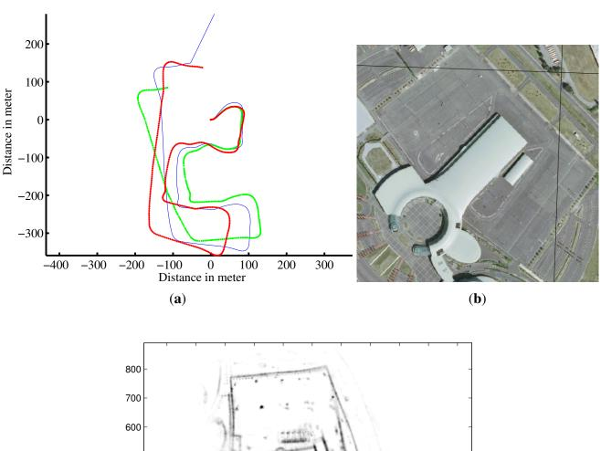
**Figure 11.** Trajectory and map reconstruction based on IMPALA radar odometry. (a) Estimated trajectory with IMPALA odometry: in blue the ground truth, in red the reconstructed trajectory with the measurements of the odometer and gyrometer, and in green radar-odometry solution; (b) Aerial view of the experimental area; (c) Map obtained based on radar odometry with the estimated velocities.
