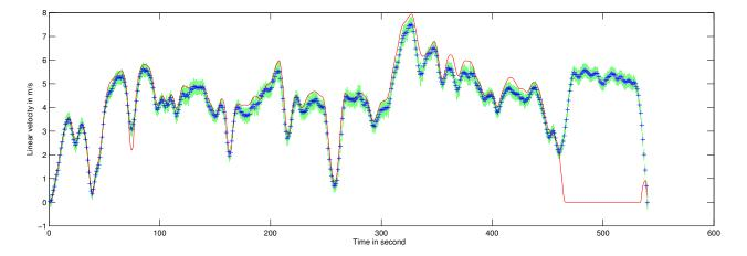
**Figure 15.** Estimation of velocities by the IMPALA radar-based odometry approach. (a) and (b) represent the linear and angular velocity estimates respectively. Ground truth velocity obtained by D-GPS and odometer is in red. In blue are the estimates given by the method.
