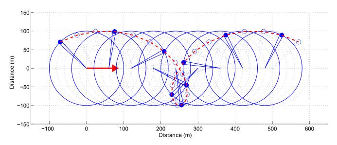
As regards some other displacements of the center of rotation, the distortion equation can be represented by the parametric equation of a trochoid. Indeed, at time t, the position of a detection done at range  $\rho$  is a function of the center pose  $(x_t^c, y_t^c, \phi_t^c)$  and of sensor bearing  $\theta_t$ .
