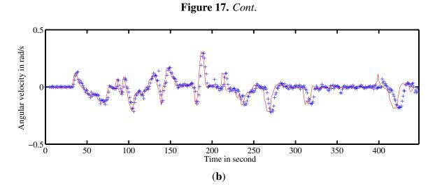
**Figure 18.** Estimation of velocities. (a) and (b) represent the linear and angular velocity estimates respectively. Ground truth velocity is in red. The estimates given by the method are in blue.
