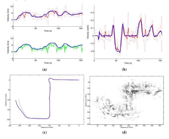
**Figure 21.** IMPALA odometry results in dynamic environment. (a) Linear velocity estimation: in blue the ground truth plotted on the two graphs, in green the Doppler estimation and in red the odometry estimation, both plotted with their respective uncertainty; (b) Angular velocity estimation (in red) along with ground truth (c) Estimated trajectories: in red the IMPALA odometry and in blue the ground truth; (d) Map obtained based on the trajectory solution.
