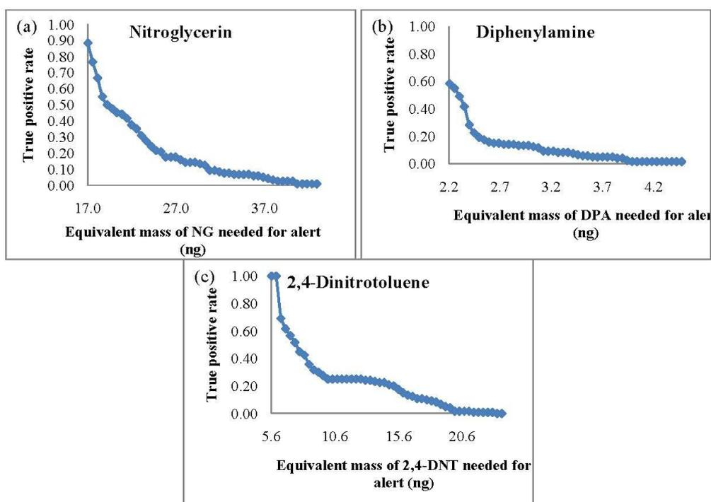
In comparison to the PSPME-IMS studies, SPME-GC-MS led to poorer sensitivity with a TPR of 0.88 and a minimum detection of 17 ng for NG and a TPR of 1.0 with equivalent mass detection of 6 ng for 2,4-DNT. Detection of DPA was slightly better with a TPR of 0.58 with detection equivalent to 2 ng of
