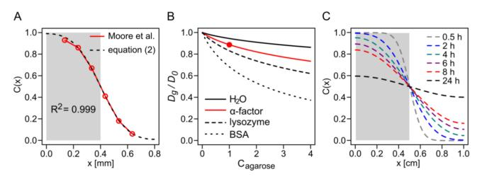
Naturally, the diffusion coefficient of molecules decreases with the increase of agarose concentration (Figure S3B). The model was applied to four different molecules: water,  $\alpha$ -factor, and two proteins of well-known hydrodynamic radius, lysozyme ( $R_H = 1.9$  nm) and bovine serum albumin (BSA,  $R_H = 3.5$  nm) [4]. The impact on the diffusion coefficient is stronger for molecules with larger
