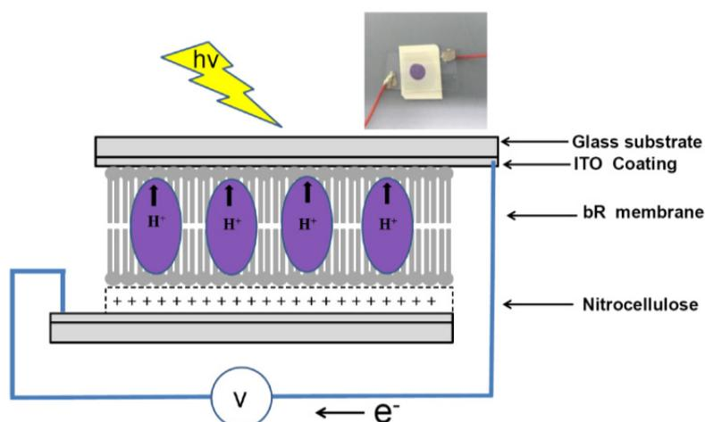
The cell was made by 1.5 cm<sup>2</sup> nitrocellulose membrane (PNM) placed on top of a 2 cm<sup>2</sup> ITO coated glass. Purified PM (20 μL, 1.2 mg/mL) was deposited on the top of the PNM and dried at room temperature. Both ITO electrodes were connected to electronic instruments to measure the PM/PNM properties.
