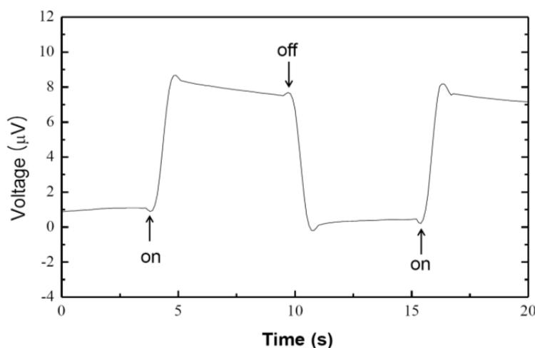
**Figure 3.** Photoinduced current from PM/PNM as a function of illumination time. The peak wavelength of incident light was 537 nm.
