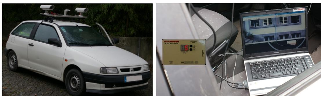
Twenty traffic signs distributed in urban and near urban areas, were surveyed with GNSS differential static methods. The accuracy of those measurements is expected at centimeter level. With the described MMS mounted on a vehicle this traffic signs were surveyed when at distances between 10 and 45 meters. Differences with the GNSS coordinates were calculated and are presented in Table 4, together with the mean and the RMSE.
