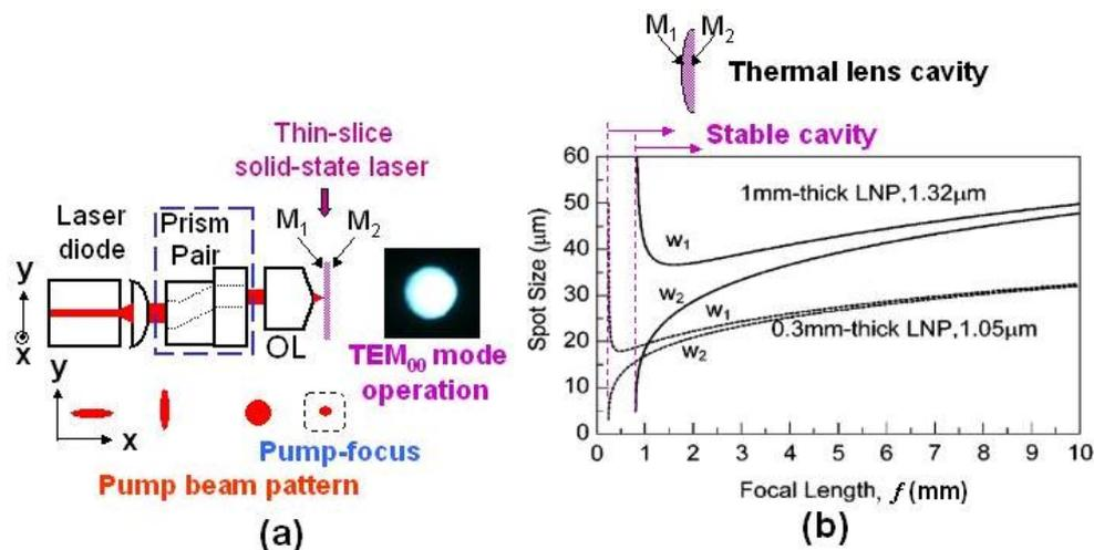
The thin-slice laser consists of a platelet laser crystal with mirrors coated on end surfaces ( $M_1$ : anti-reflection at pump wavelength and 99.9% reflection at lasing wavelength;  $M_2$ : 99% reflection at lasing wavelength).
