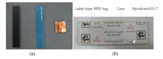
We tested the detecting range with ALR-9800 RFID-Reader, because we needed to estimate the optimum thickness of Styrofoam 103.7 before the comparison of a proposed structure with the commercial units.
