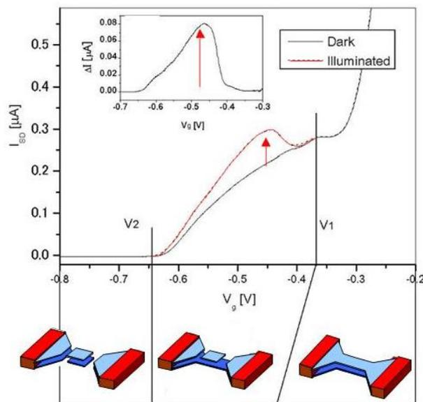
This photoresponse can be interpreted by increase of electron density in lower QW induced by capacitively coupled photoholes stored in the isolated upper QW. The unit increment of current  $I_e$  induced by one photohole in the isolated upper QW (area of  $L \times W$ ) is given by [17,22]:
