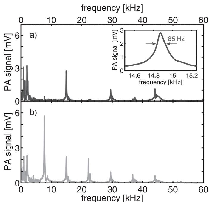
By measuring the peak value of the 2nd longitudinal resonance at 14.87 kHz as a function of gas flow, it was found out that the peak amplitude of the PA signal increases. This is probably due to the
