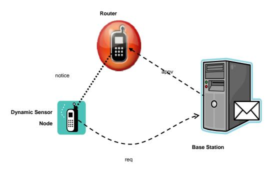
After receiving the *req* message, the base station will check its revocation list whether the sensor node has been revoked. If the sensor node is acceptable, then the base station verifies the MAC message. If the result is positive, the base station will generate a session key  $K_{NR}$  for the roaming sensor node and the router (or cluster head).
