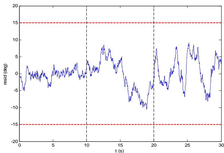
The residuals are obtained as the difference between the signals, and a CUSUM filter with forgetting factor is used to analyze them. Figure 4 shows the residual of the comparison between the virtual sensor angle estimate (GVIRT) and the wing angle derived from the actuator command
