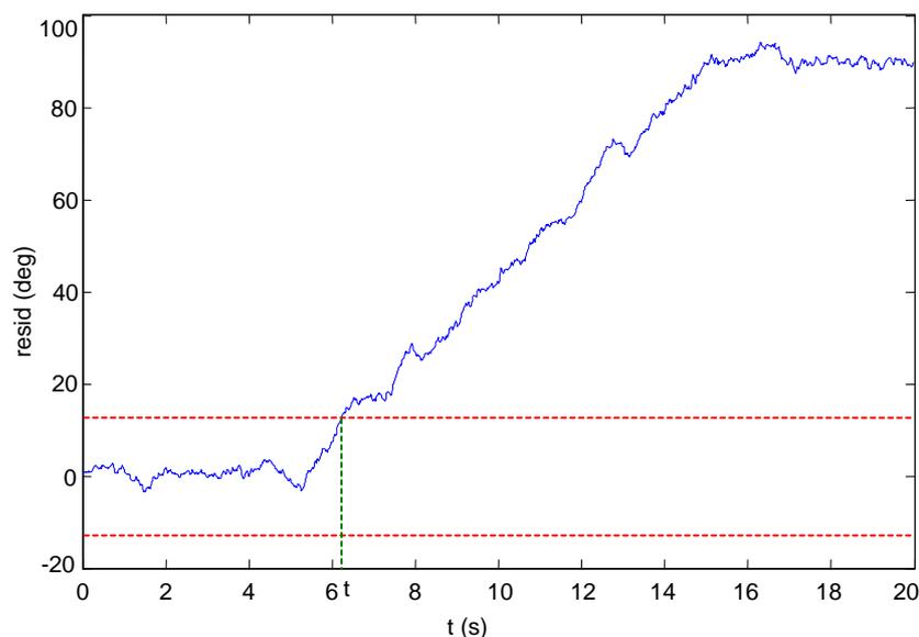
The actuator is instructed to unfold the wings at constant angular velocity between  $t = 5$  s. and  $t = 15$  s. It can be seen that the residual error begins to grow after the command, and goes above the threshold level, since the virtual sensor GVIRT detects that the actuator has not moved the wings but
