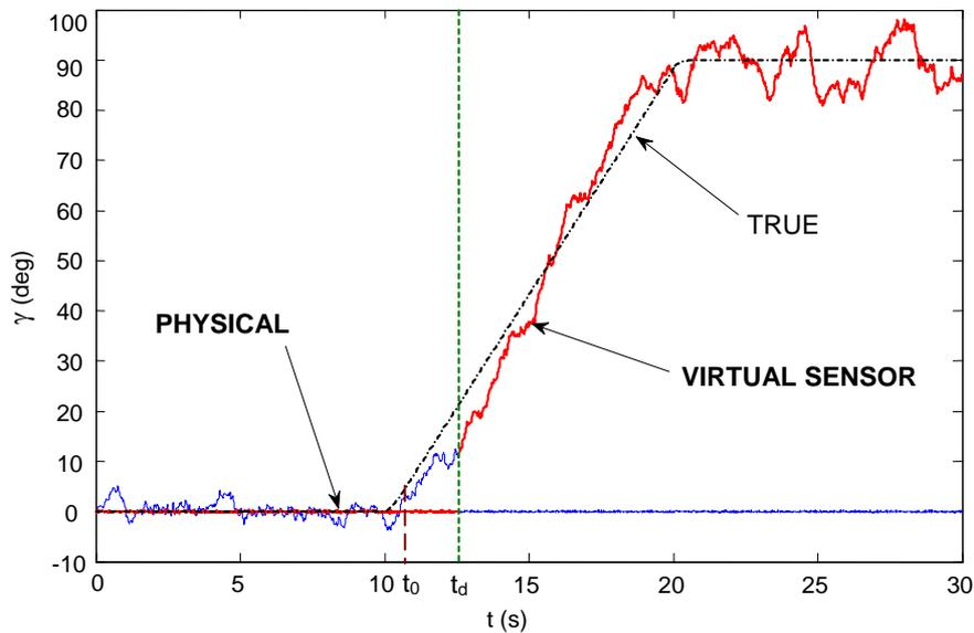
In the same way, if the residual of GVIRT and GSENS do not grow larger than the threshold value it can be considered that the fault is located at the actuator and not the angle sensor.
