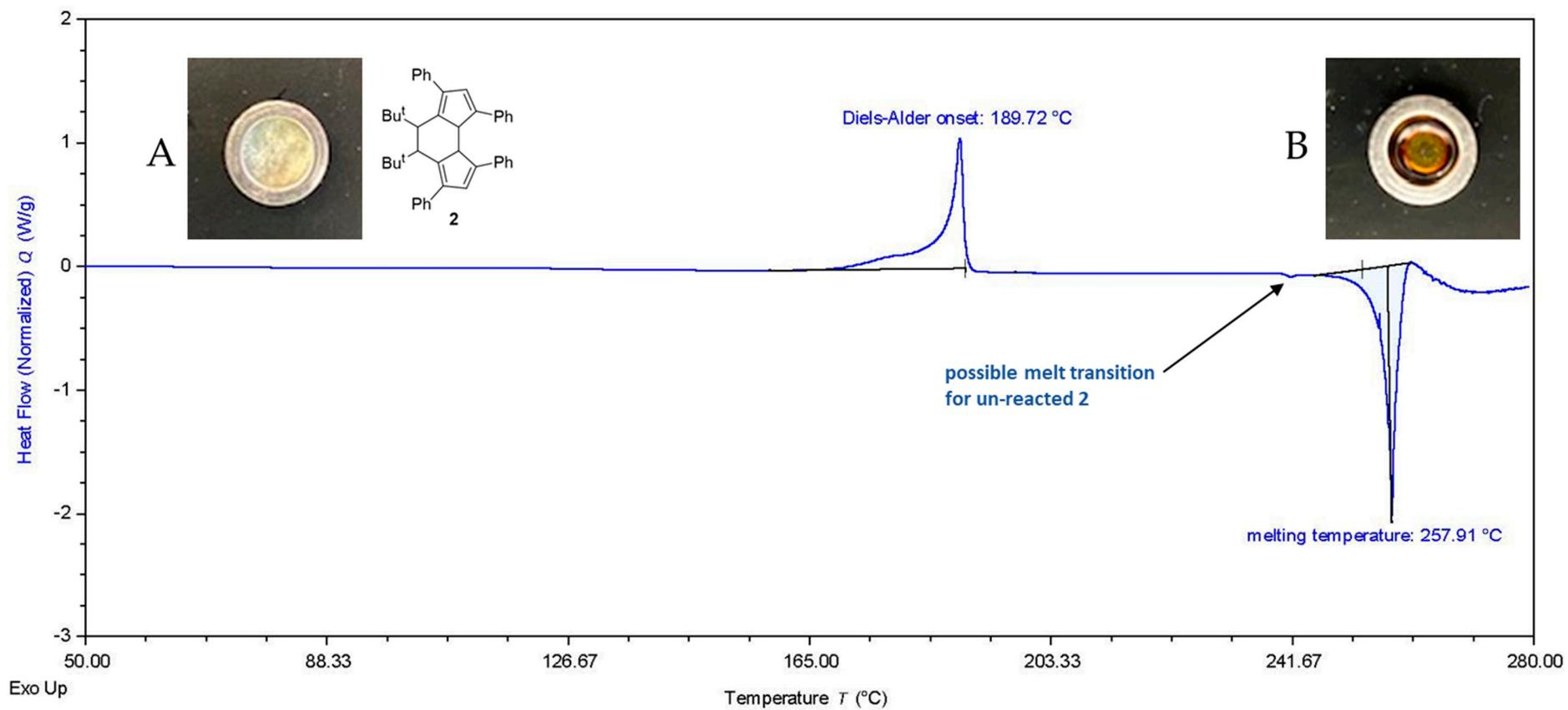
Figure S9. DSC thermogram of **2** (crystalline sample from iPrOH under  $\text{N}_2$ , open Al pan, ambient to 280 $^{\circ}$  C, 5 $^{\circ}$  C/min). Insets show appearance of a powdered sample of **2** in Al pan at the beginning of the analysis (photo A), and dark brown appearance of residue after melting and some decomposition (photo B).
