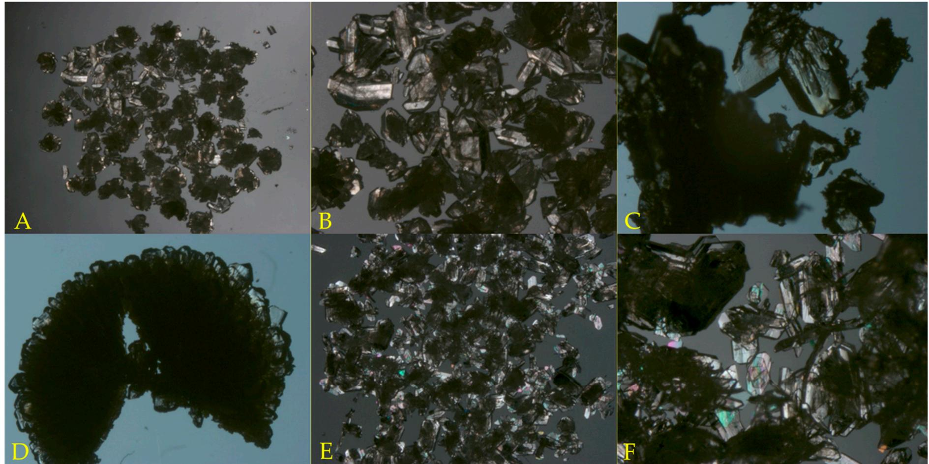
Figure S12. Microscopic images of crystalline samples of **2** taken under polarized transmitted light. Crystals from iPrOH (A), iPrOH magnified view (B), 50/50 THF/MeOH magnified view (C), 50/50 THF/MeOH MeCN layer (D), 2-butanol (E), 2-butanol magnified view (F). Images were taken using a Zeiss Stereo Discovery V12 stereomicroscope.
