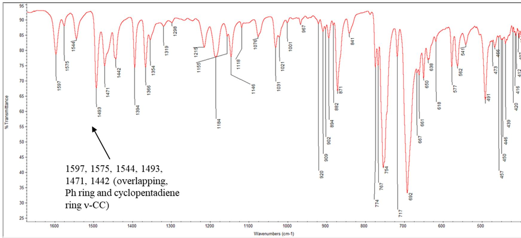
Figure S5A. Expansion of the FTIR spectrum of crystalline **2** (ATR). The crystalline sample of **2** was obtained from hot iPrOH by slow cooling and evaporation.
