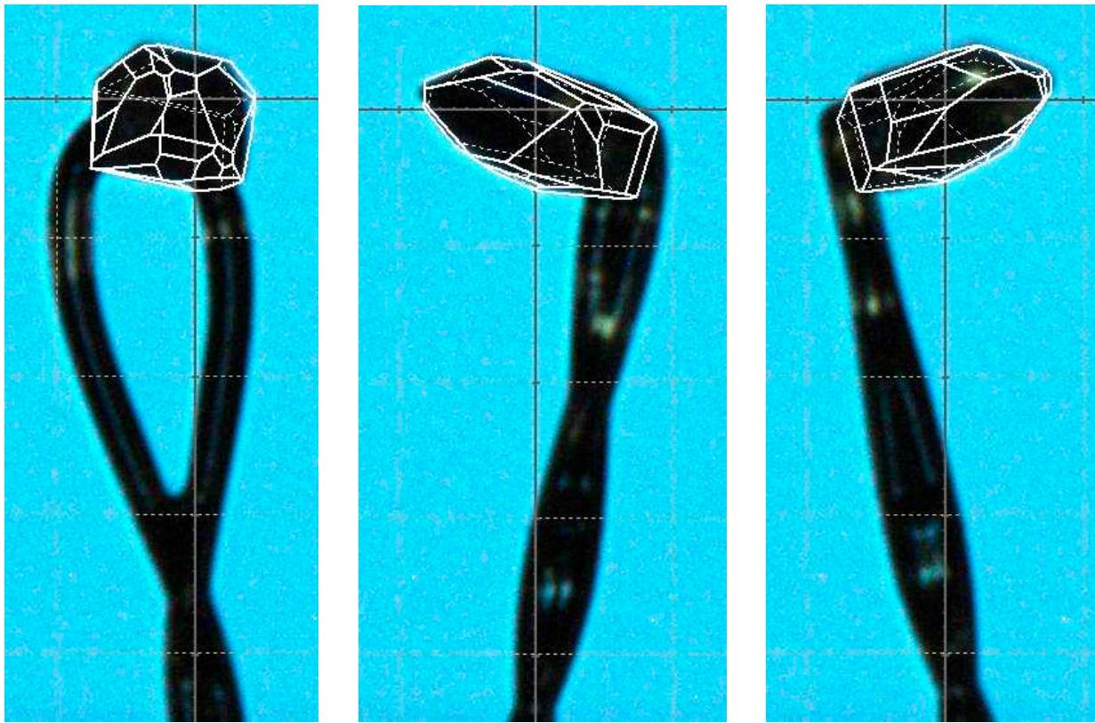
Figure S23. Images of the mounted crystal of **2** (THInd2ABS, crystal from 2-butanol solution). A  $0.181 \times 0.115 \times 0.082 \text{ mm}^3$  translucent colorless prism crystal was selected from crystals that were grown from a hot 2- butanol solution by slow cooling and evaporation.
