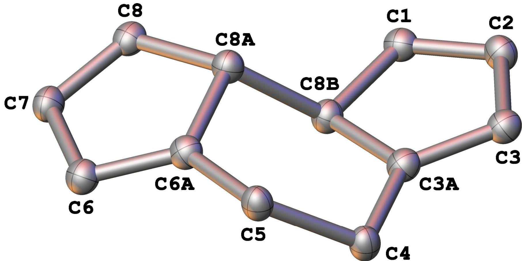
Figure S14. Thermal ellipsoid view of the core structure of **2**, showing two cyclopentadiene rings fused to a central 6–membered ring. Ph groups, Bu<sup>t</sup> groups and H atoms were omitted for clarity. Thermal ellipsoids are shown at the 50% probability level.
