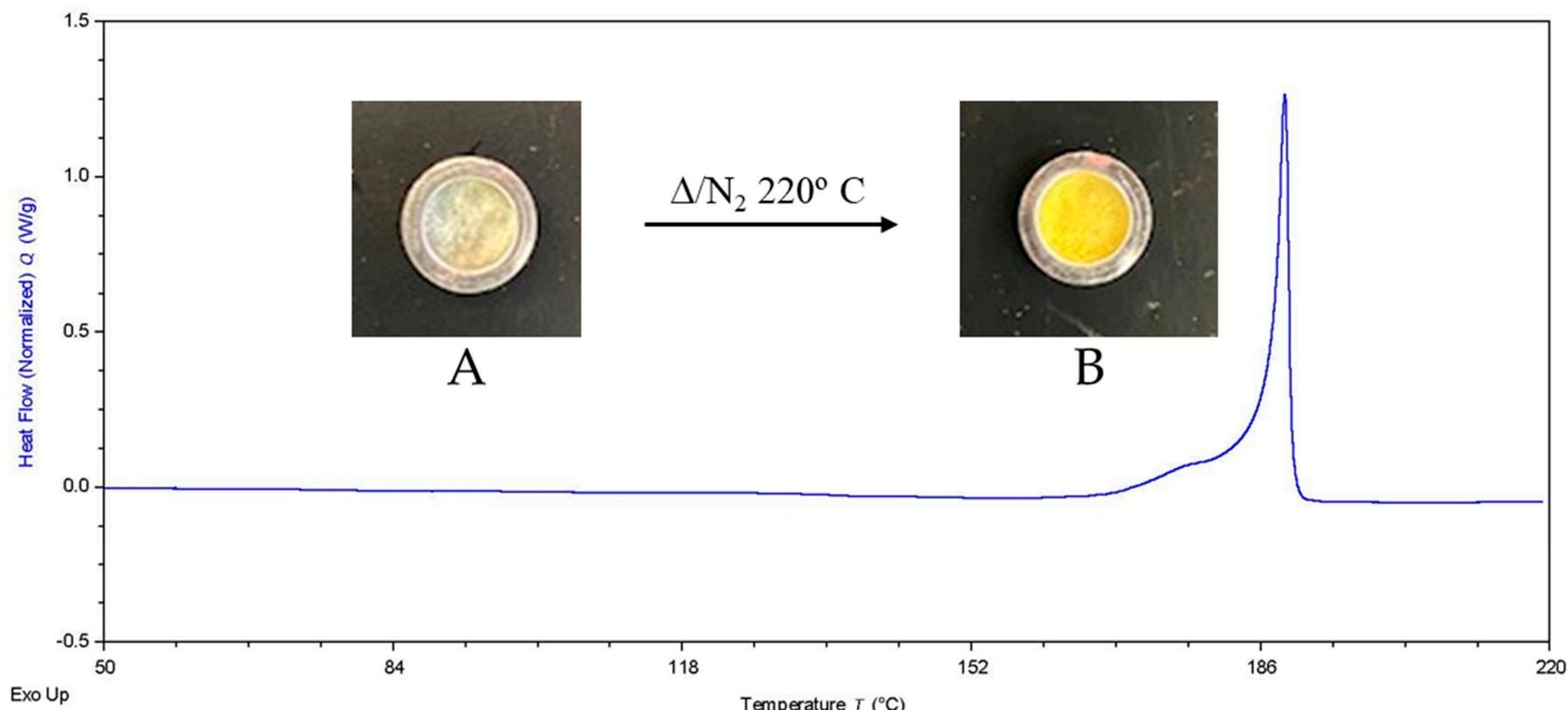
Figure S10. DSC thermogram of **2** (crystalline sample from iPrOH under N<sub>2</sub>, open Al pan, ambient to 220° C, 5° C/min). Insets show appearance of a powdered sample of **2** in Al pan at the beginning of the analysis (photo A), and yellow appearance of residue from conversion of **2** to a possible Diels-Alder adduct (photo B).
