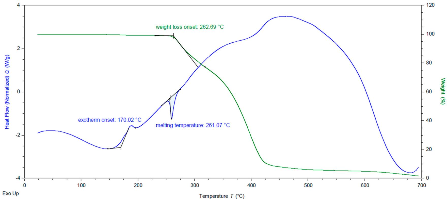
Figure S8. SDT thermogram of **2** (crystalline sample from iPrOH under N<sub>2</sub>, ambient to 700° C, 10° C/min).
