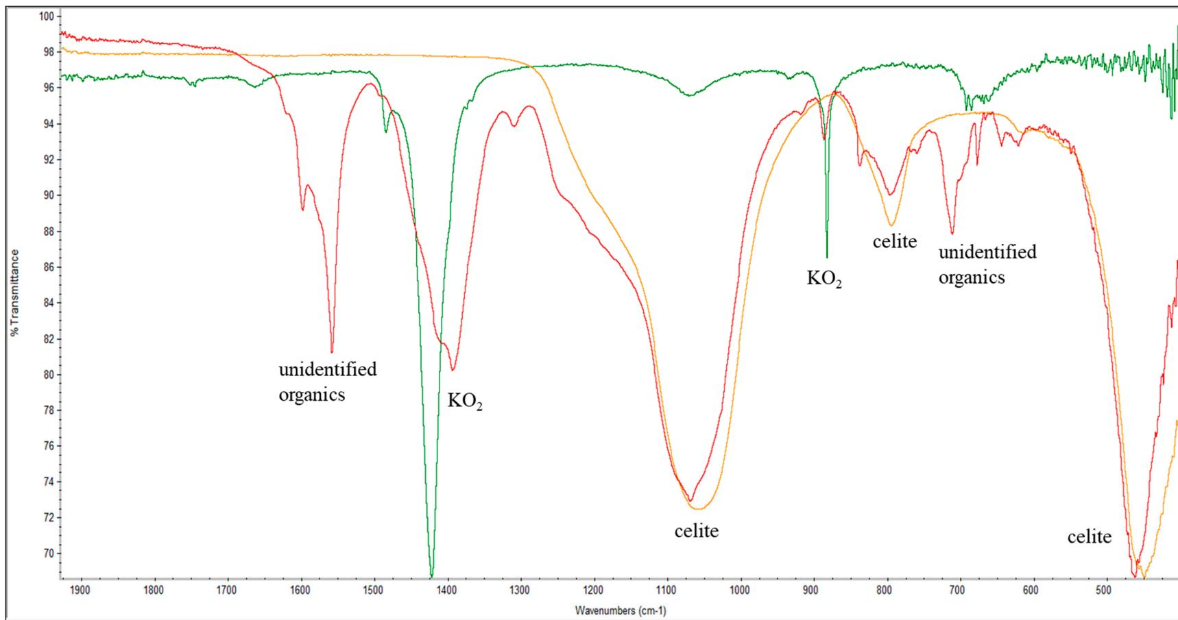
Figure S7. Overlay of the FTIR (ATR) spectra ( $400 - 1900 \text{ cm}^{-1}$ ) of the dry filtered by-product contaminated with celite (red spectrum), authentic  $\text{KO}_2$  (green spectrum) and celite (orange spectrum), showing presence of  $\text{KO}_2$  in the by-product.
