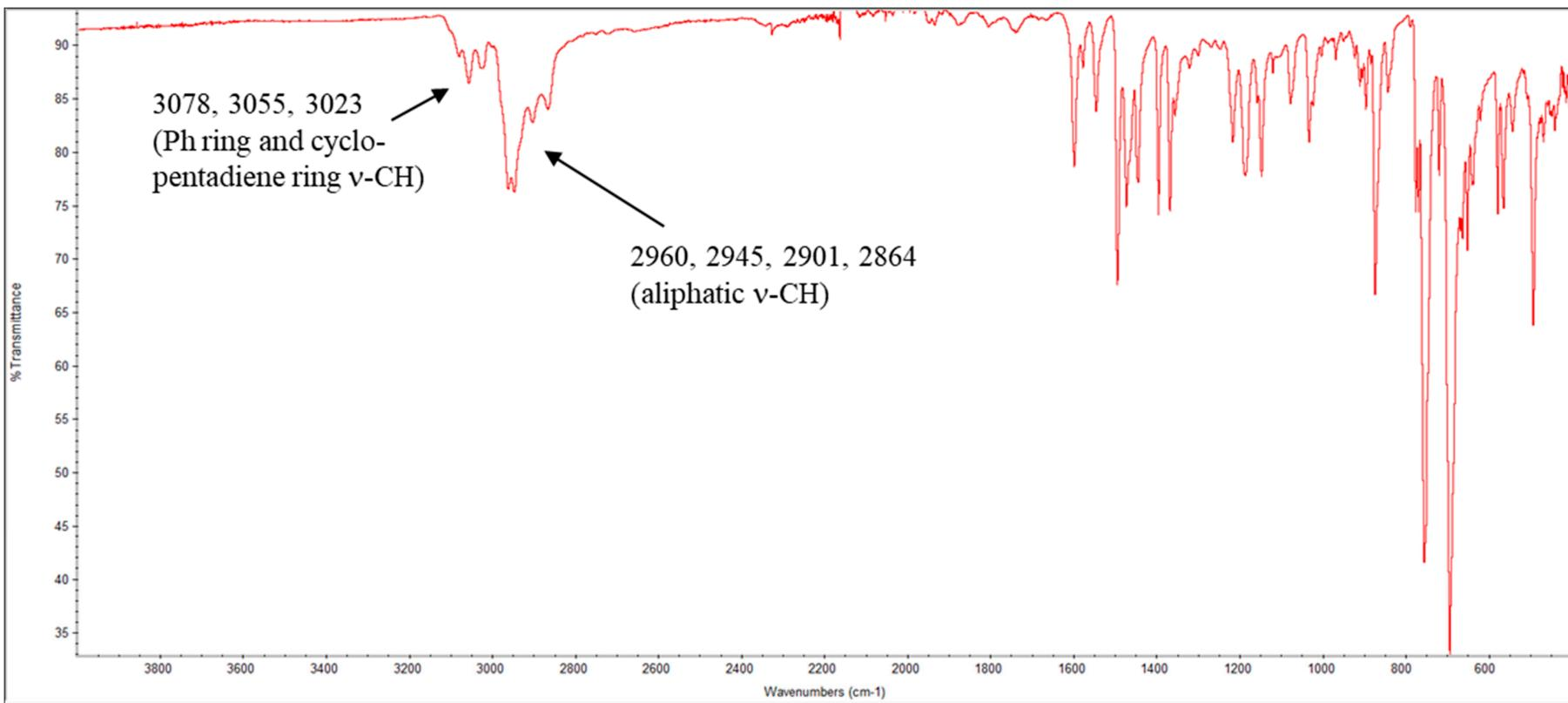
Figure S5. FTIR spectrum of crystalline **2** (ATR). The crystalline sample of **2** was obtained from hot iPrOH by slow cooling and evaporation.
