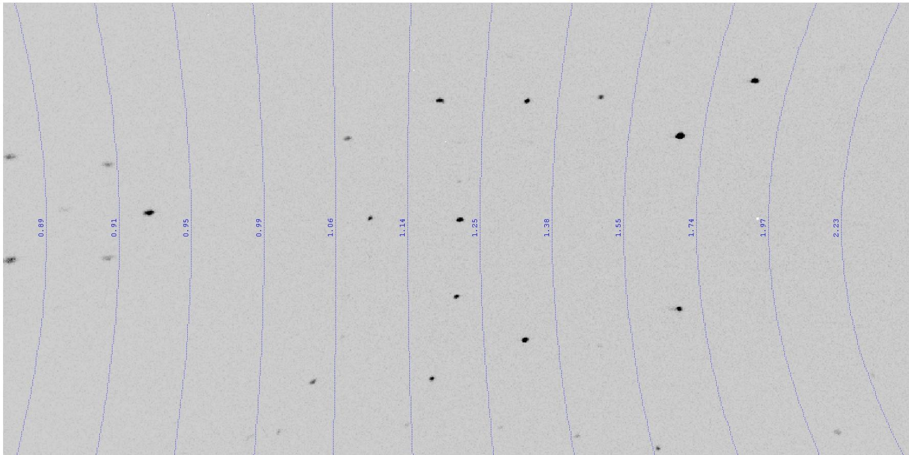
Figure S18. Example frame taken from the series of runs (run 4, frame 66), demonstrating excellent diffraction for the selected crystal of **2** (THInd1ABS).
