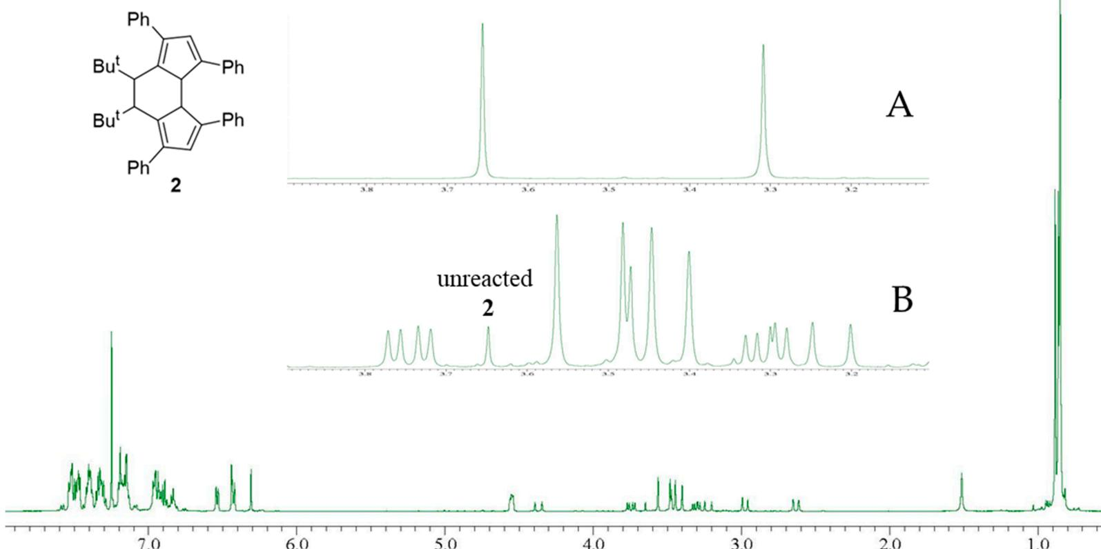
Figure S11.  $^1\text{H}$  NMR spectrum of yellow residue in DSC pan after pyrolysis of **2** (in  $\text{CDCl}_3$ , crystalline sample from iPrOH, open Al pan, ambient to  $220^\circ\text{ C}$ ,  $5^\circ\text{ C}/\text{min}$ ), indicating formation of a possible Diels-Alder adduct. Comparison of an expansion of the  $^1\text{H}$  NMR spectrum of pure **2** (A) with that of the yellow converted product (B) shows some un-converted **2** after pyrolysis to  $220^\circ\text{ C}$ .
