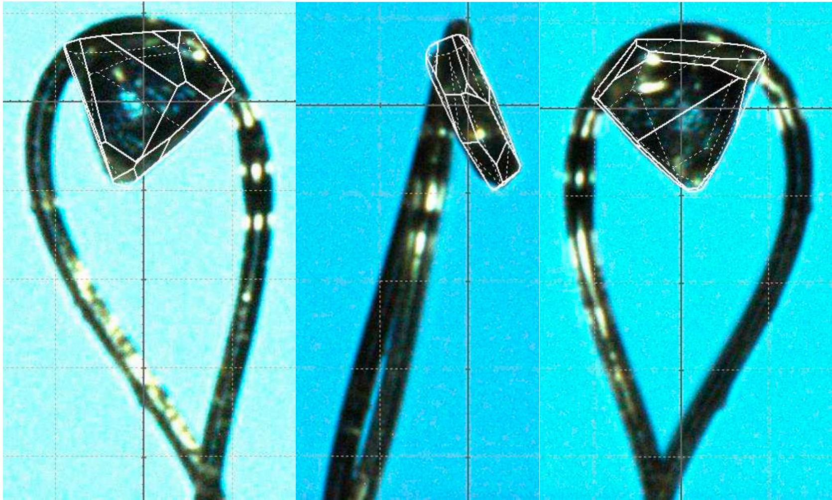
Figure S17. Images of the mounted crystal of **2** (THInd1ABS). A  $0.184 \times 0.164 \times 0.055 \text{ mm}^3$  translucent colorless prism crystal was selected from crystals that were grown from a hot iPrOH solution by slow cooling and evaporation.
