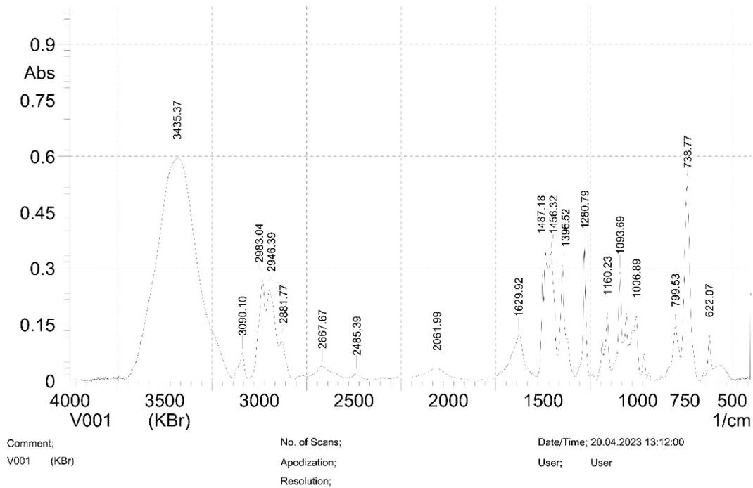
Figure S7. FTIR spectrum of 2, KBr.
