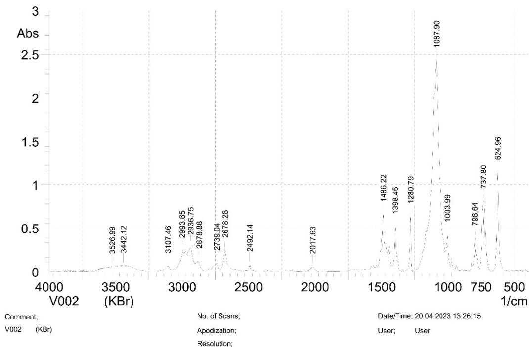
Figure S8. FTIR spectrum of 3, KBr.
