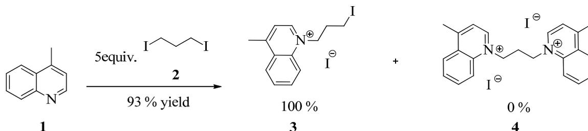
**Scheme 1.** Preparation of 1-(3-iodopropyl)-4-methylquinolin-1-ium iodide **3**.
