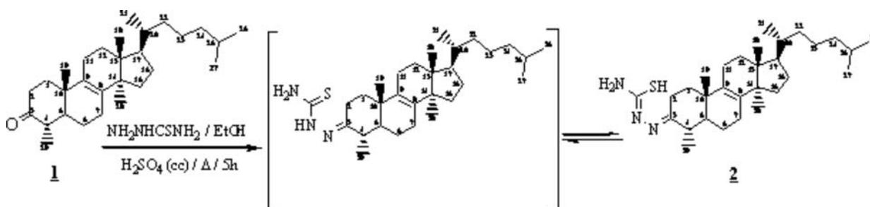
The compound **2** was prepared from equimolar quantity of **1** (1g, 2.43 mmol), derivative triterpene resulting from *Euphorbia officinarum*<sup>1</sup>, and thiosemicarbazide<sup>2,3</sup> dissolved in ethanol with several drops of conc. H<sub>2</sub>SO<sub>4</sub>. The mixture was heated at reflux for 5h, and evaporated under reduced pressure. The residue was purified on silica gel column using hexane: ethyl acetate (90:10) as eluent yielded compound **2** (0.99g, 2.06mmol) in 85% yield.
