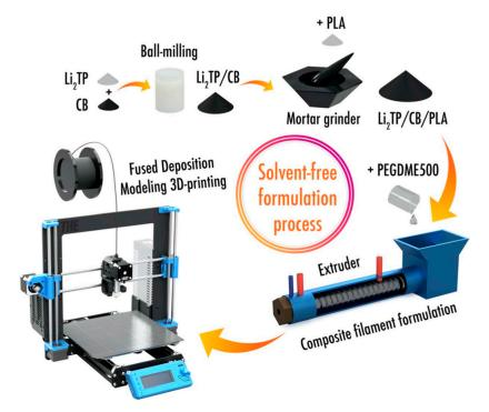
**Figure 4.** Solvent-free formulation process of a corn-based PLA-containing filament for the 3D printing of a lithium-ion battery [117]. Reproduced with permission (Copyright 2021 The Electrochemical Society, under CC BY 4.0).
