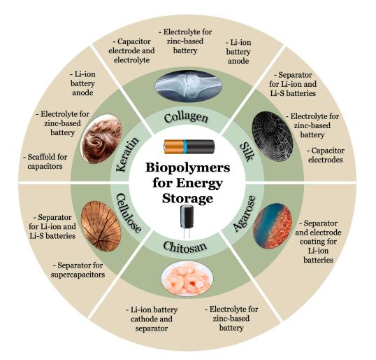
**Figure 2.** Source and applications for biopolymers commonly utilized for energy storage purposes such as batteries and capacitors. Keratin, collagen, and silk are protein-based biopolymers while cellulose, chitosan, and agarose are polysaccharide-based biopolymers. (Images of biopolymers were obtained with permission from pixabay.com, accessed on 1 December 2022).
