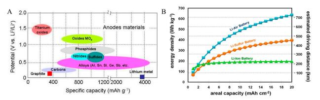
**Figure 1.** (**A**) The electric potential and specific capacity of various anode materials [49]. (**B**) Plot of energy density ( $W \cdot h \cdot g^{-1}$ ) vs. areal capacity ( $mA \cdot h \cdot cm^{-2}$ ) for three distinct anodes. Energy density is also displayed in terms of a theoretical driving distance if these batteries were used in an electrical vehicle [50]. Reproduced with permissions ((**A**). Copyright AIMS Press 2016 under CC BY 4.0; (**B**). Copyright 2014 Springer Nature).
