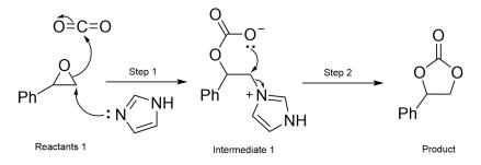
**Scheme 2.** Proposed reaction mechanism for the Lewis base catalysed cycloaddition of  $CO_2$  into SO to form SC. Imidazole is taken as representative example for all the Lewis base catalysts of this study.
