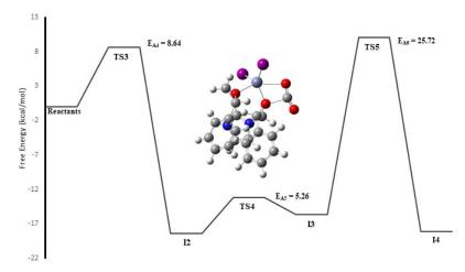
**Figure 11.** Free energy diagram (kcal/mol) of HIm/ZnI<sub>2</sub> catalyzed transformation of styrene oxide (SO) to styrene carbonate (SC).
