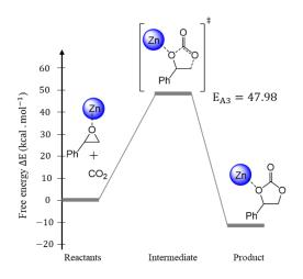
Figure 9. Free energy diagram (kcal/mol) of ZnI<sub>2</sub> catalyzed transformation of SO to SC.
