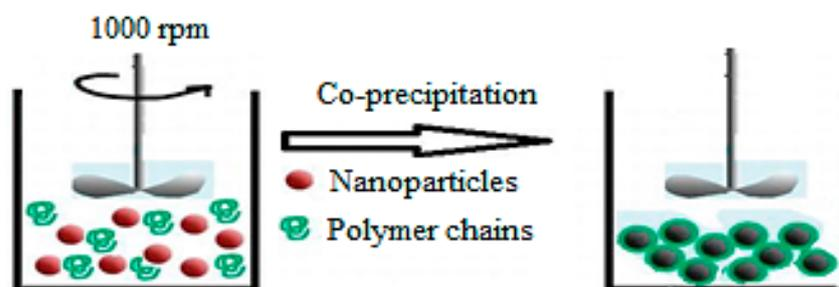
**Figure 2.** Schematic illustration for the solution mixing method (taken from [27]).
