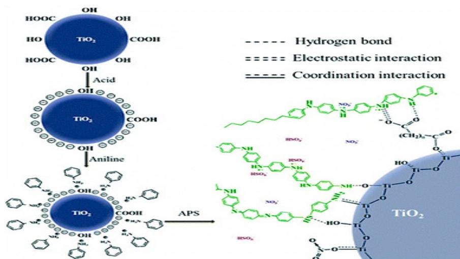
**Figure 9.** Schematic representation of the adsorption mechanisms by polyaniline/TiO<sub>2</sub> nanocomposite (taken from [89]).
