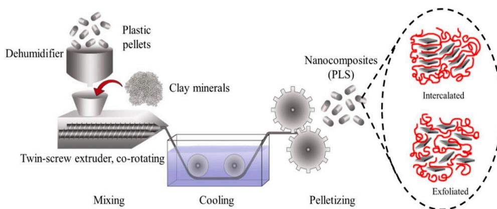
**Figure 3.** Schematic representation for preparing polymer nanocomposites by melt blending (taken from [37]).
