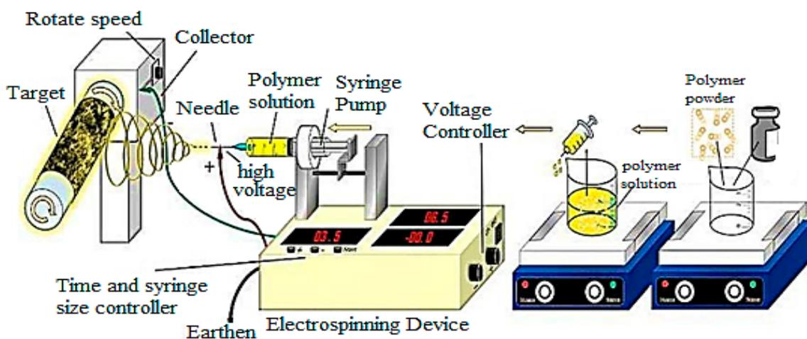
Figure 4. The set-up of electrospinning technique (taken from [45]).
