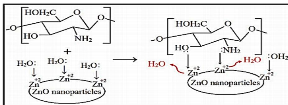
**Figure 5.** Complexation reaction between chitosan functional groups and  $Zn^{+2}$  ions of ZnO nanoparticles (taken from [46]).
