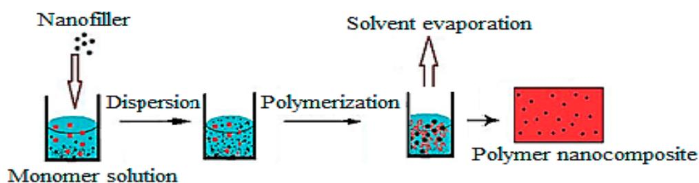
**Figure 1.** Schematic illustration for the in situ polymerization method (taken from [27]).
