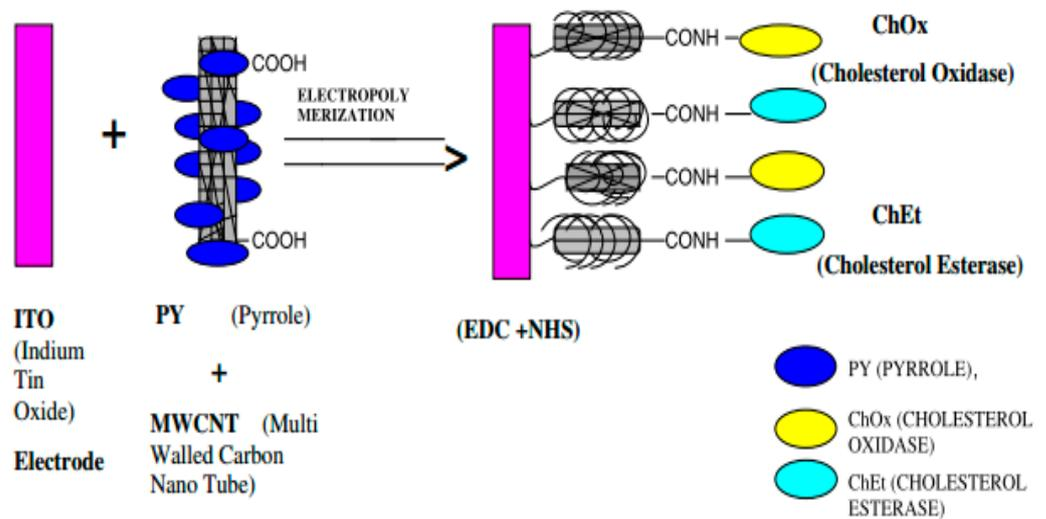
Figure 12. Fabrication of nanocomposite electrode (taken from [138]).
