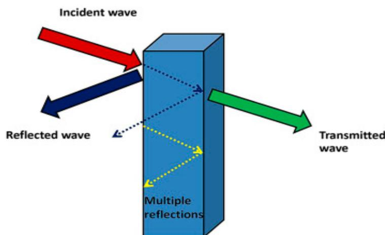
Figure 13. Schematic representation of EMI shielding (taken from [164]).
