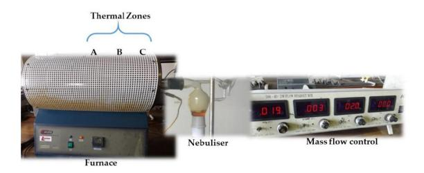
Figure S3. CVD set-up of the synthesis of VA-MWCNTs.
