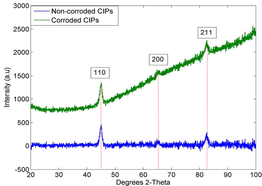
**Figure 3.** XRD patterns for corroded and non-corroded CIPs.
