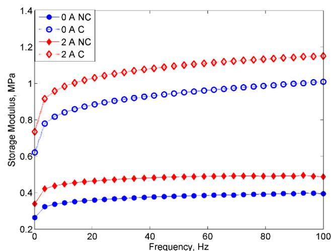
**Figure 6.** Storage modulus vs. frequency for MRE with non-corroded (NC) and corroded (C) CIPs at off- and on-state conditions.
