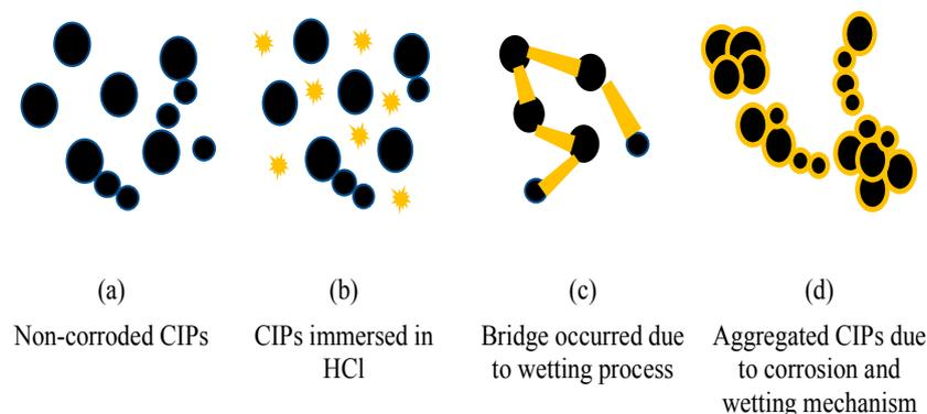
**Figure 11.** Mechanism of aggregated CIPs due to the corrosion process are illustrated in (a) Non-corroded CIPs, (b) CIPs immersed in HCl, (c) Bridge occurred due to wetting process and (d) Aggregated CIPs due to corrosion and wetting mechanism.
