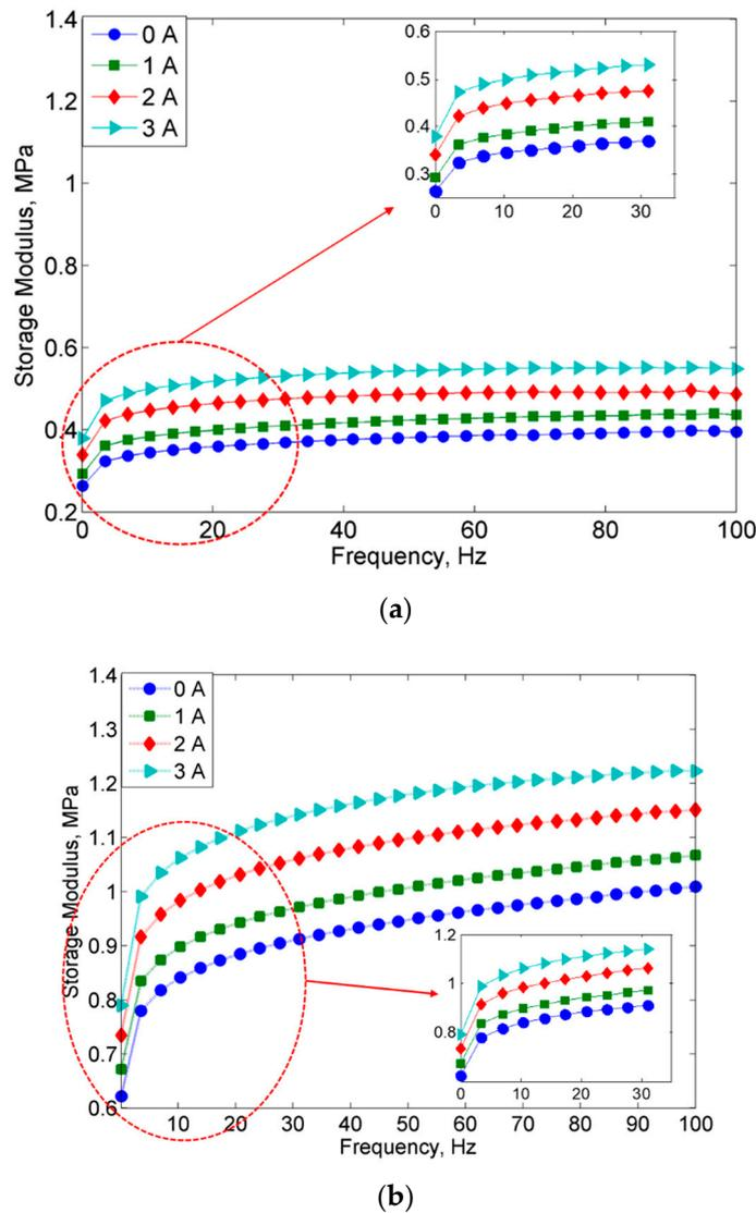
**Figure 5.** Storage modulus vs. frequency of (a) MRE with non-corroded CIPs and (b) MRE with corroded CIPs at different applied currents.
