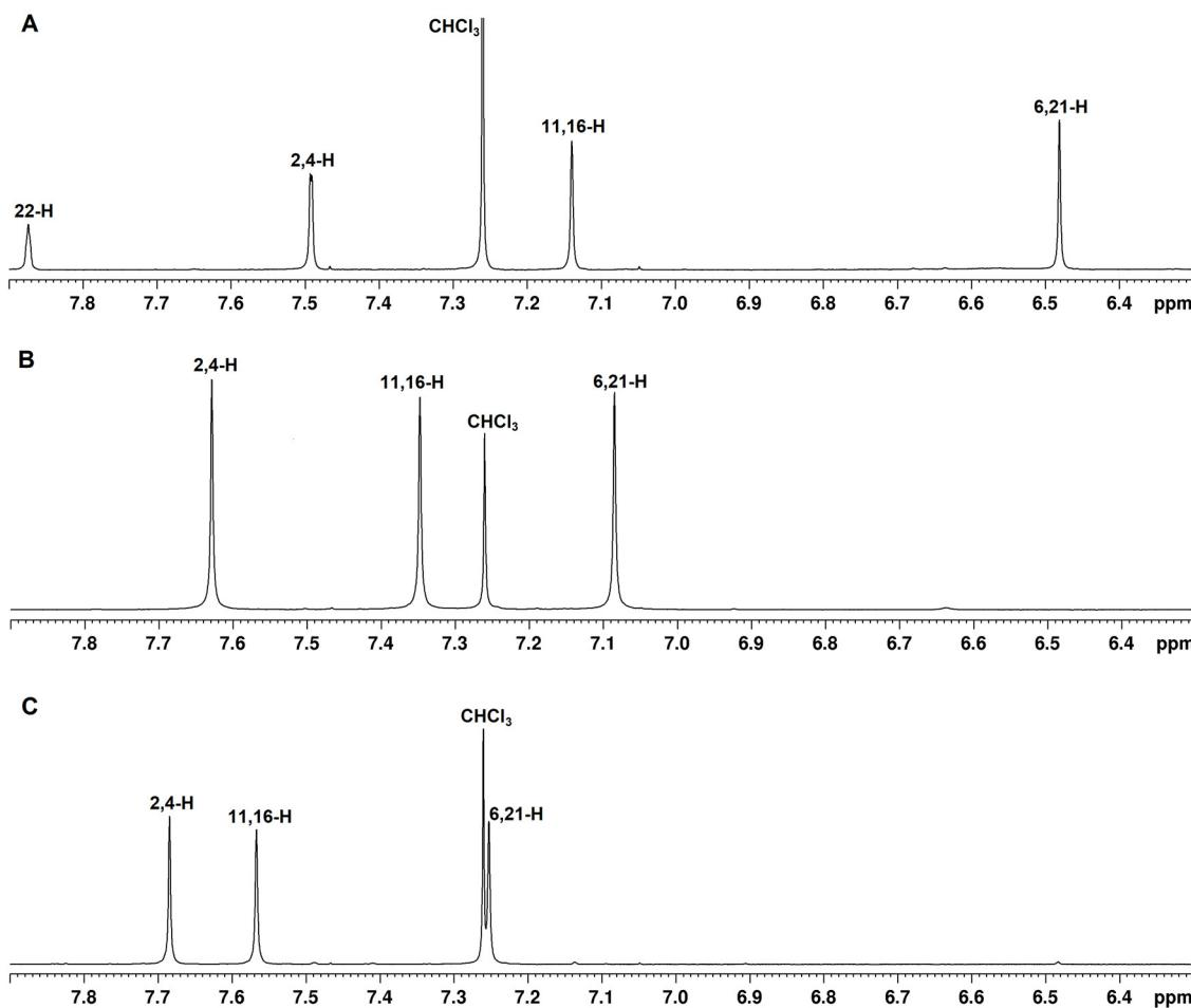
**Figure 4.** Partial proton NMR spectra of methoxybenzoporphyrin **7a** (A) and the related nickel(II) complex **7aNi** (B) and palladium(II) complex **7aPd** (C) showing a marked increase in diatropicity upon metalation, which was most pronounced for **7aPd**.
