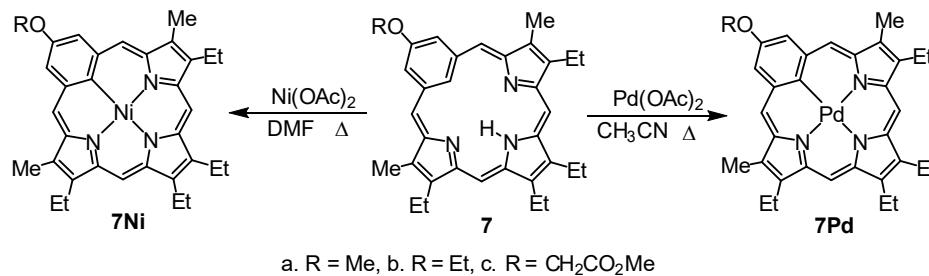
**Scheme 4.** Metalation of 3-alkoxybenzoporphyrins.
