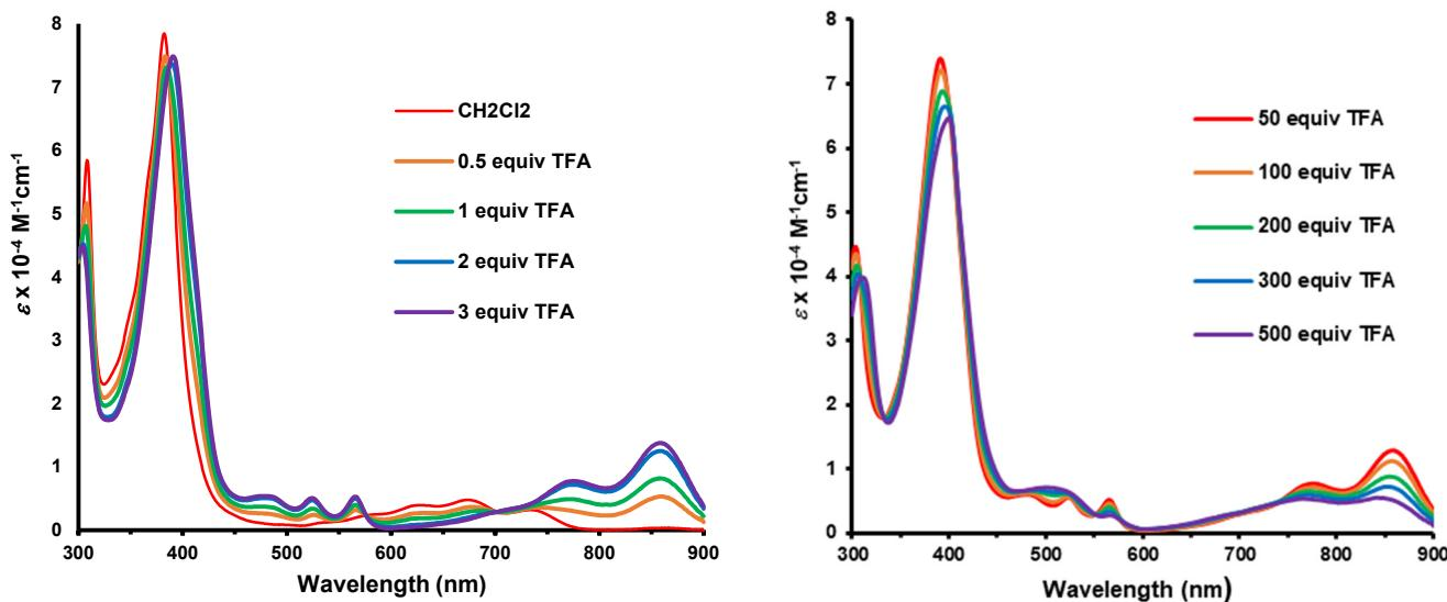
**Figure 3.** UV-vis spectra of ethoxybenzoporphyrin **7b** in dichloromethane with 0–3 equivalents of TFA (**left**) and 50–500 equivalents of TFA (**right**) showing sequential mono- and diprotonation.
