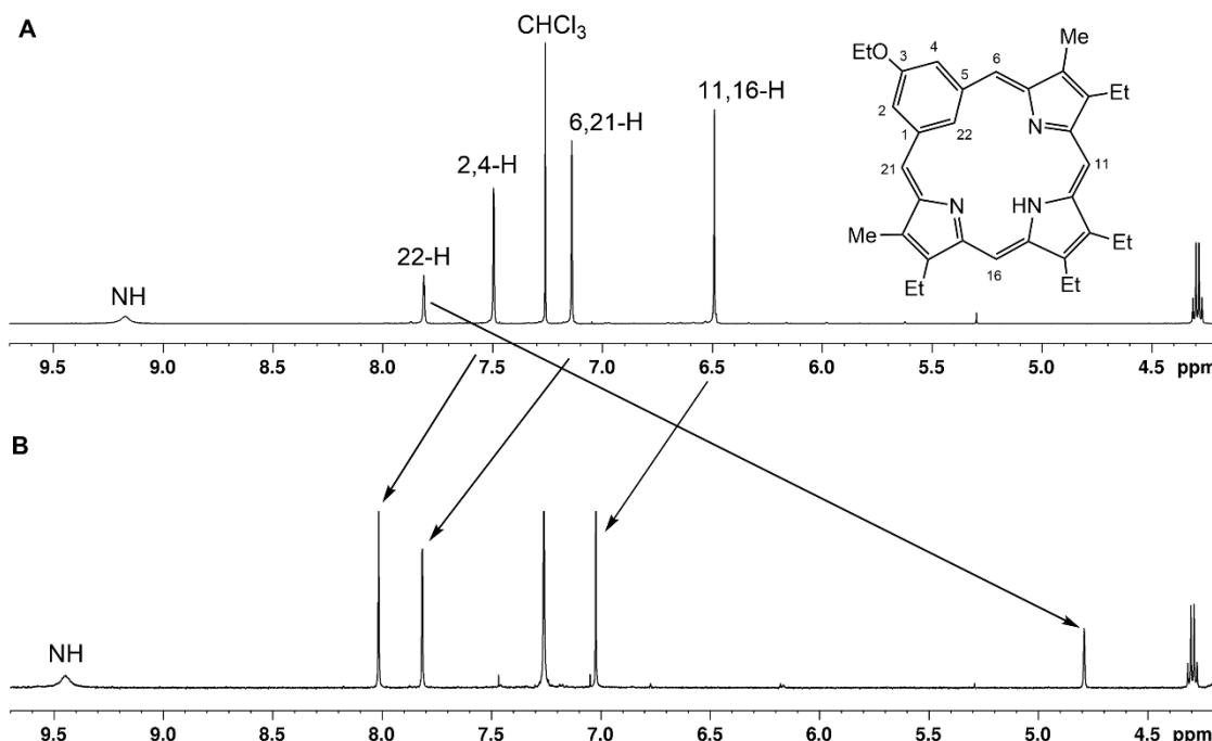
**Figure 2.** Partial 500 MHz proton NMR spectra of ethoxybenzoporphyrin **7b** in  $\text{CDCl}_3$  (**A**) and the related diprotonated dication in TFA- $\text{CDCl}_3$  (**B**). Protonation leads to the internal 22-H shifting upfield by ca. 3 ppm while the external protons are significantly deshielded, results that demonstrate the emergence of a global aromatic ring current.
