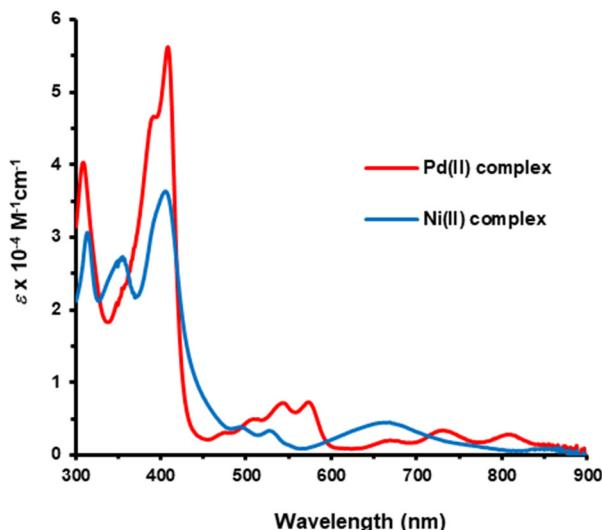
**Figure 5.** UV-vis spectra of **7aNi** (blue) and **7aPd** (red) in  $\text{CH}_2\text{Cl}_2$ .
