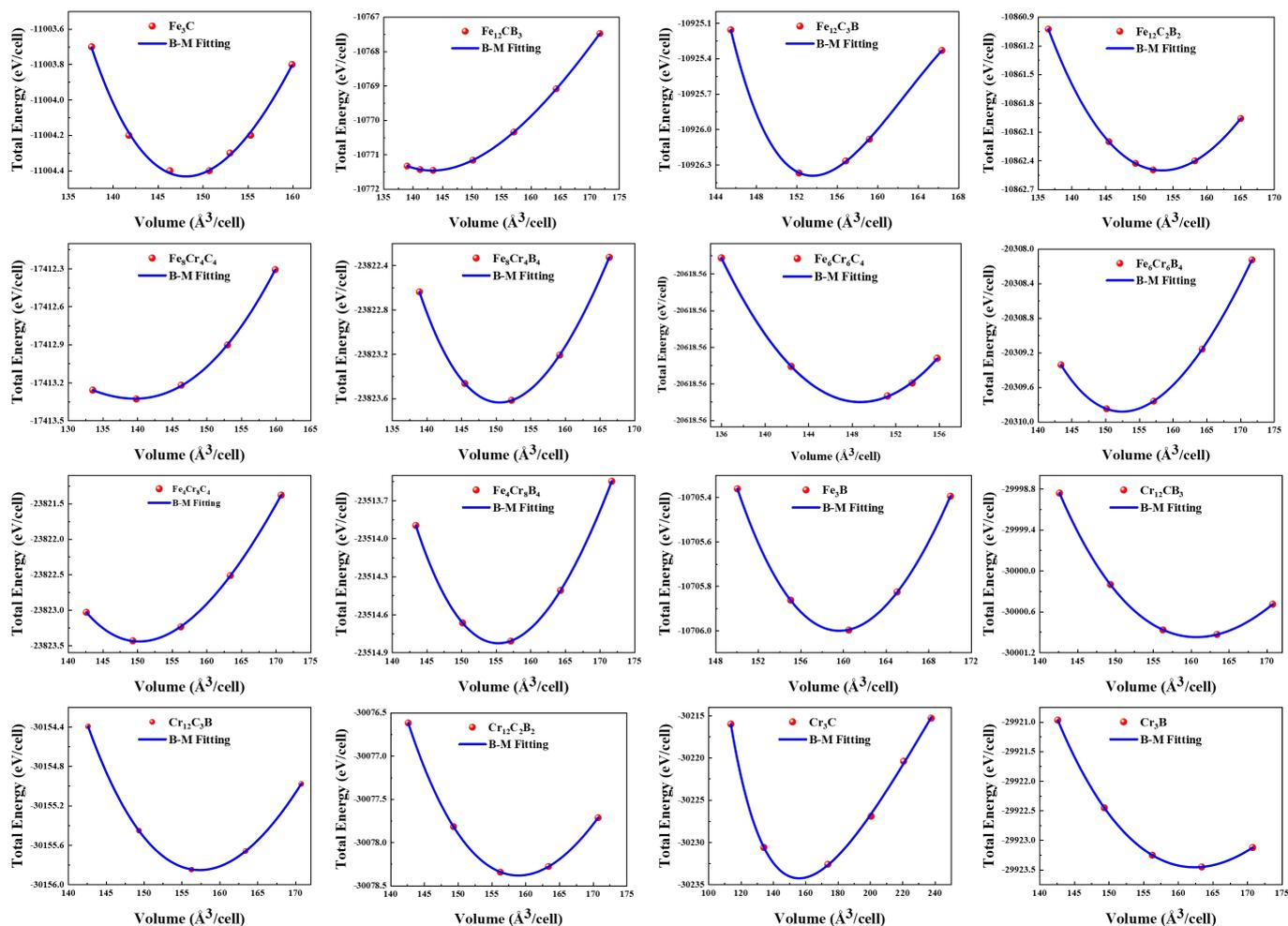
**Figure 3.** Calculated total energy at zero temperature and without zero point motion as a function of volume of  $M_3X$  ( $M = Fe, Cr$ ;  $X = C, B$ ). The filled circles represent calculated points, and the line is a fit to EOS in Equation (1).
