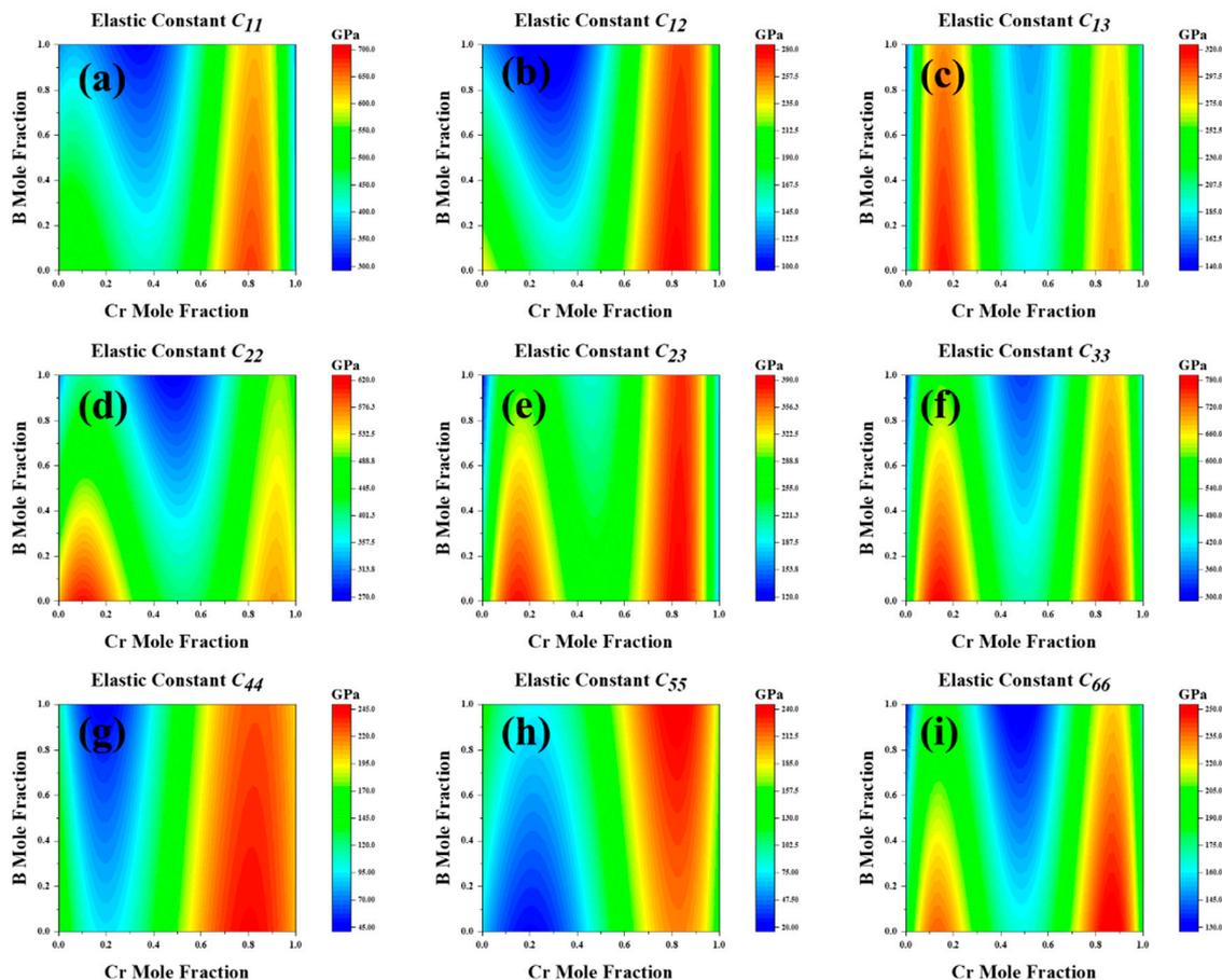
**Figure 6.** The elastic constants over the whole composition space of cementite-type  $\text{M}_3\text{X}$  ( $\text{M} = \text{Fe}, \text{Cr}$ ;  $\text{X} = \text{C}, \text{B}$ ). (a)  $C_{11}$ , (b)  $C_{12}$ , (c)  $C_{13}$ , (d)  $C_{22}$ , (e)  $C_{23}$ , (f)  $C_{33}$ , (g)  $C_{44}$  (h)  $C_{55}$ , (i)  $C_{66}$ .
