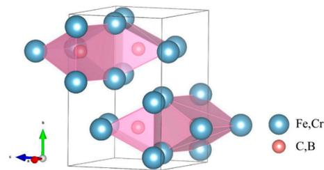
**Figure 1.** The crystal structure of cementite-type  $\text{M}_3\text{X}$  shows the orthorhombic space lattice, where blue represents the positions of metal atoms and red represents the positions of non-metal atoms.
