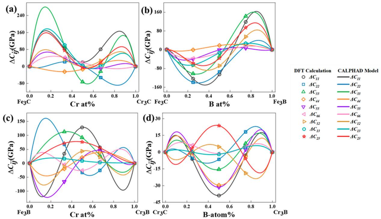
**Figure 4.** The elastic constants of cementite-type  $M_3X$  ( $M = \text{Fe, Cr}; X = \text{C, B}$ ) calculated by DFT and fitted by CALPHAD model. (a)  $(\text{Fe,Cr})_3\text{C}$ , (b)  $\text{Fe}_3(\text{C,B})$ , (c)  $(\text{Fe,Cr})_3\text{B}$  and (d)  $\text{Cr}_3(\text{C,B})$ .
