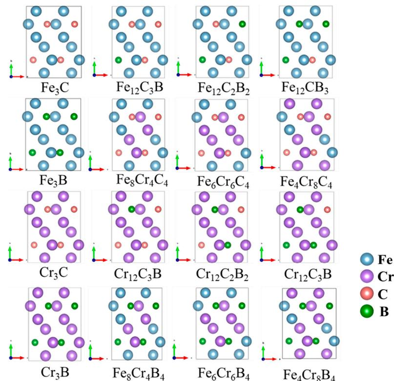
**Figure 2.** The atomic configurations of Fe, Cr, B and C in a unit cell of  $(\text{Fe, Cr})_3(\text{C, B})$ , consisting of formula units (16 atoms). The purple and blue spheres correspond to Fe and Cr atoms, while the red and green spheres represent B and C atoms.
