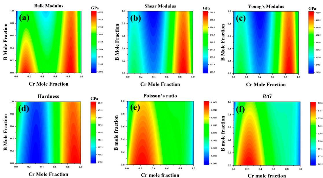
**Figure 7.** The elastic modulus over the whole composition space of cementite-type  $M_3X$  ( $M = \text{Fe, Cr}$ ;  $X = \text{C, B}$ ). (a) the bulk modulus ( $B$ ), (b) shear modulus ( $G$ ), (c) Young's modulus ( $E$ ), (d) hardness ( $Hv$ ), (e) Poisson's ratio ( $\nu$ ), (f)  $B/G$ .
