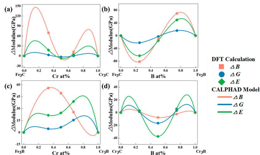
**Figure 5.** The elastic of modulus cementite-type  $M_3X$  ( $M = \text{Fe}, \text{Cr}; X = \text{C}, \text{B}$ ) calculated by DFT and fitted by CALPHAD model. (a)  $(\text{Fe,Cr})_3\text{C}$ , (b)  $\text{Fe}_3(\text{C,B})$ , (c)  $(\text{Fe,Cr})_3\text{B}$  and (d)  $\text{Cr}_3(\text{C,B})$ .
