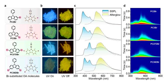
**Figure 2.** Designing organic afterglow molecules through the direct population of triplet excited states. (a) Br-substituted organic afterglow molecules with corresponding single-crystal structures; (b) photographs before (**left**) and after (**right**) 365 nm excitation; (c) SSPL and organic afterglow emission spectra; and (d) transient PL decay images excited by 295 nm light at room temperature.
