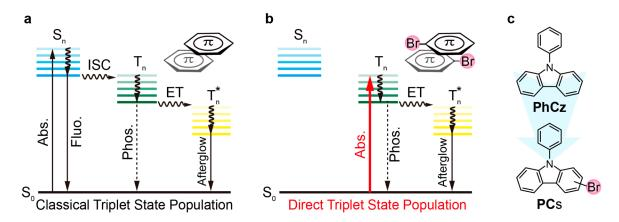
**Figure 1.** Two distinct approaches to achieve organic afterglow. (a) The traditional mechanism; (b) direct population of the  $T_1$  state through intra/intermolecular heavy-atom effect-induced  $S_0 \rightarrow T_1$  absorption; and (c) the corresponding molecular design strategy.
