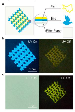
**Figure 4.** Color-encoded and excitation wavelength-dependent pattern encryption. (a) Device structure of the flexible pattern encryption. Photographs of the device under (b) 365 nm UV and (c) white LED irradiation (left), as well as after the removal of the excitation (right).
