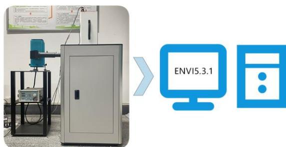
**Figure 9.** Fluorescence hyperspectral system.
