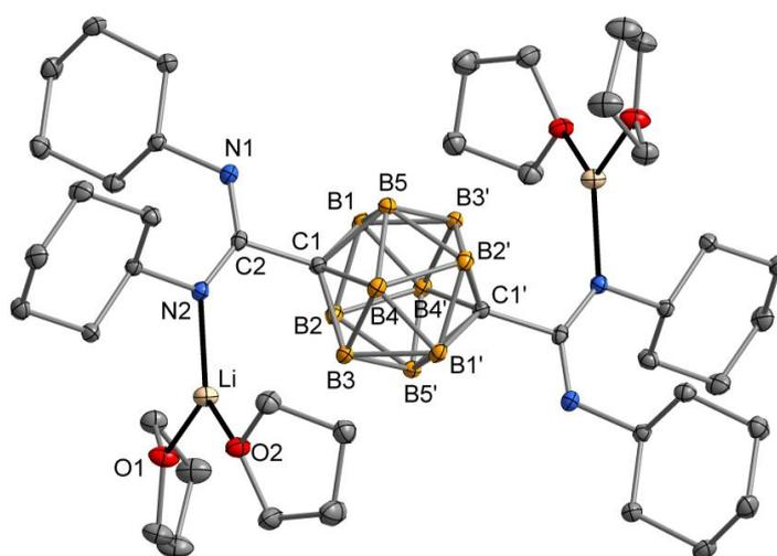
**Figure 2.** Molecular structure of 3 in the crystal. Displacement ellipsoids of the heavier atoms are drawn with 50% probability; H atoms are omitted for clarity. Selected bond lengths (Å) and angles (deg.): C(1)–C(2) 1.551(2), N(1)–C(2) 1.305(2), N(2)–C(2) 1.340(2), N(2)–Li 1.953(3), O(1)–Li 1.949(3), O(2)–Li 1.933(3), N(1)–C(2)–N(2) 136.9(1), N(1)–C(2)–C(1) 109.7(1), N(2)–C(2)–C(1) 113.4(1), C(2)–N(2)–Li 134.9(1). Symmetry code to generate equivalent atoms:  $2-x, 1-y, 1-z$ .
